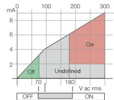
\* The threshold may be between Vmaxoff and Vminion Ioff is defined at the threshold
