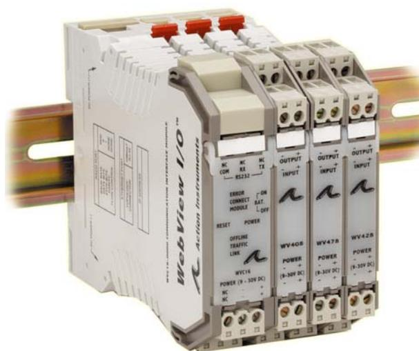
DC power also needs to be connected to the unit. Apply 9 to 30VDC to the WVC16 either through the power clips (the red and black clips supplied with each module) or hard-wire DC Power (+) to terminal 11 or 21 and DC Power (-) to terminal 12 or 22.
