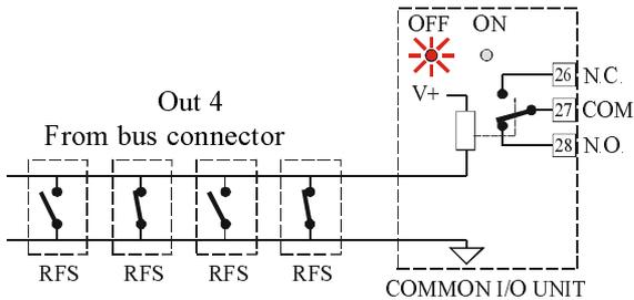
Fig. 20/B Relay energized, beacon OFF lit.
