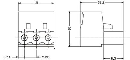
Fig. 22 - 3 wires connector
