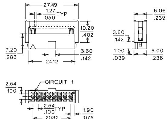
**Fig. 15 – CONNECTOR 8 x 2 FOR BUS CABLE
