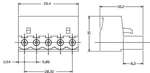
Fig. 24 - 5 wires connector
