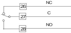
Fig. 19 COMMON ALARM OUTPUT WIRING
