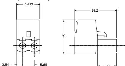
Fig 21 – 2 wires connector
