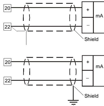
Fig. 6.A mA INPUT WIRING
