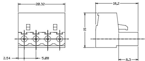
Fig. 23 - 4 wires connector
