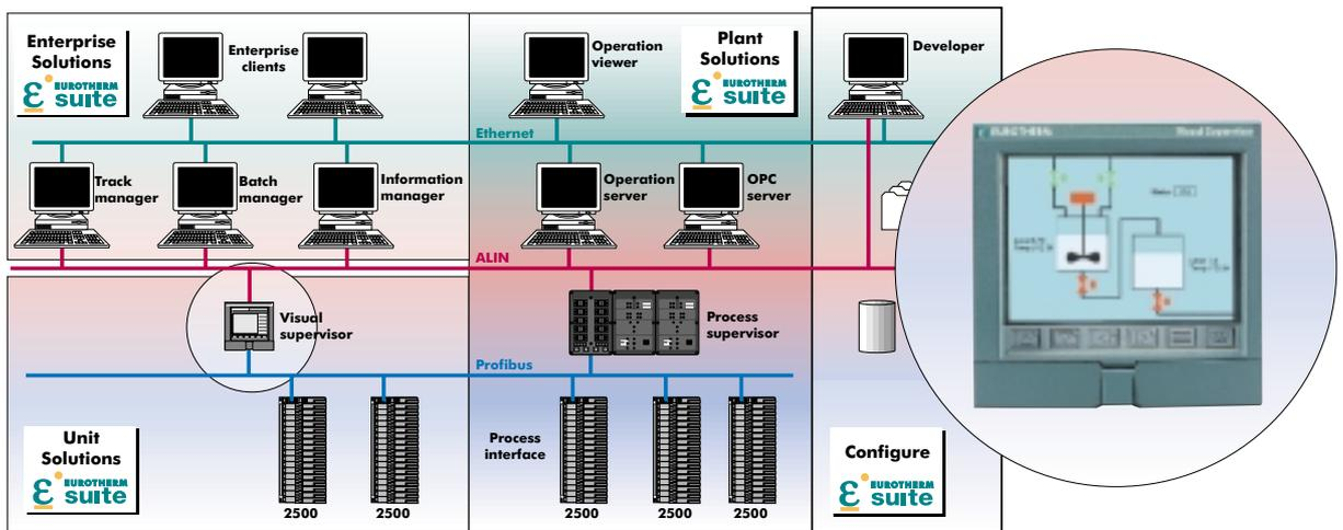
The Visual Supervisor is a combined operator panel and controller capable of performing both continuous and sequential control. It features comprehensive alarm and event management and local data logging facilities. Evolved from a well-established range of LIN products, the Visual Supervisor can be used as a stand-alone system, or as building blocks for a larger system.
