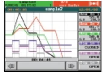
Programmes are configured from a PC using the setpoint programme editor provided with Eurotherm Project Studio. Setpoint programme editor provides multiple views of programmes, including graphical (time or segment based) and spreadsheet. Programmes can also be directly configured and edited from the Visual Supervisor. Expected and actual data can be viewed on the same display.
