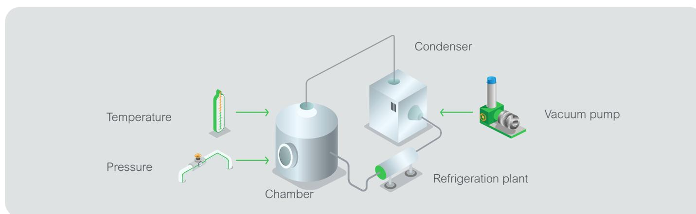
Temperature can either be controlled electrically using heating mats on the shelves, or by circulating oil through pipes welded to the shelves in the chamber. The temperature of the chamber, shelves (and/or heating oil), plus condenser form part of the control and monitoring variables also known as critical process parameters (CPPs). There are usually separate sensors for sterilization, which also require monitoring.
