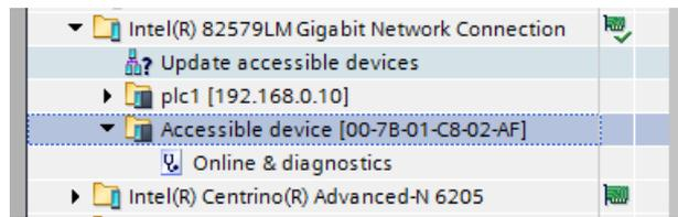
Figure 40 Example of EPack (not yet commissioned) MAC address using DCP. The next step assigns the 'IP Configuration' and the 'Device Name'. This operation can be performed by clicking on the 'Online & diagnostics' as shown in Figure 41.
