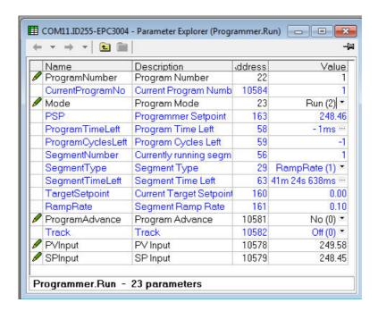
When one of the programs (Program 1 to 10) is run, the program parameters are copied into the working program. The Working Program and Working Segment parameters are then made available to the user for monitoring and/or editing.
