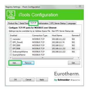
4. Click the 'Add' button to add a new connection. Type in a name of your choice, eg EPC3000, and press Add. (Ensure that no duplicate IP address entries are enabled at the same time).
