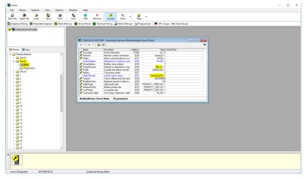
7. If the Modbus slave is online then the search result will be "Available(1)" otherwise the result will be "Unreachable(3). If it is a Eurotherm instrument with a supported profile, the "Profile" parameter will display the Modbus slave's profile otherwise it will display "3rdParty(0)".
