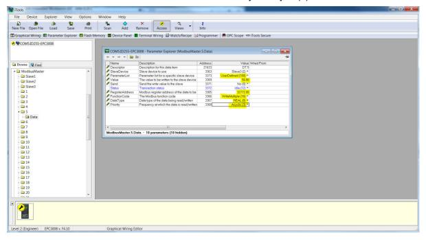
5. To send a write request, set the "Send" parameter. The Status will go to "Pending(13)" briefly before going to "Success" when the parameter has been written. If the write has failed then the Status will show the reason for the failure.
