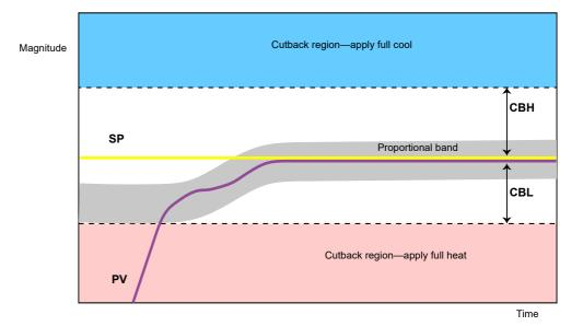
**Note:** Because cutback is a type of non-linear controller, a set of CBH and CBL values that are tuned for one particular operating point may not be satisfactory for another operating point. It is always advisable therefore not to try to tune the cutback values *too* tightly, or otherwise to use gain scheduling to schedule different values of CBH and CBL at different operating points. All the PID tuning parameters can be gain scheduled.
