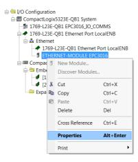
24. Set Requested Packet Interval (RPI) using Module Properties "Connection" tab making sure that it is within 50 to 3200 ms then click OK.
