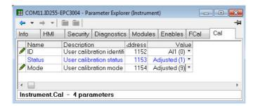
It may be found useful to open the Al1 browser list when carrying out the calibration since the PV can be read directly during the calibration procedure. This also allows the input measurement settling to be viewed during the calibration process.
