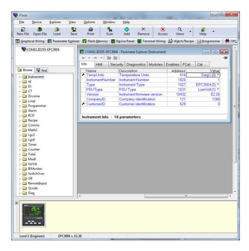
Double click on a heading to display parameters associated with the selected heading in the right hand side of the iTools view.
