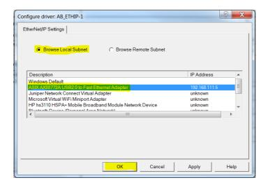
14. PC Serial and EtherNet/IP drivers must now be running. Minimize window.
