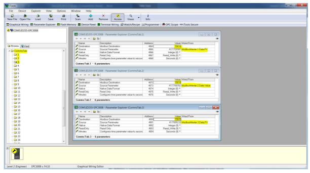
Screenshots below show Modbus Master data auto-configured to appear at the Modbus Indirection table and the values read by a 3rd party Modbus Master from our Modbus Master device:
