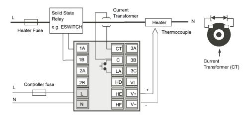
**Note:** A burden resistor value  $10\Omega$  is mounted inside the controller.
