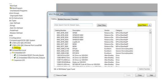
29. Filter for Eurotherm devices and then select the EPC3000 device module required (module installed in the previous section via EDS file) and then click "Create" button.
