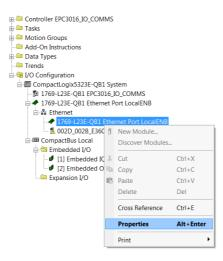
19. In the Module Properties window, configure the IP address and click OK.
