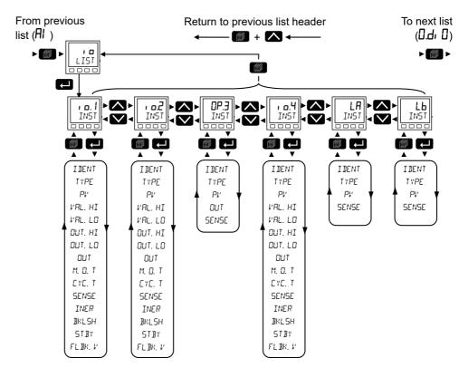
The following table includes all available input/output parameters but the ones displayed depend on how each I/O is configured.
