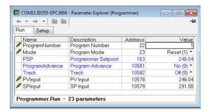
To run a program make sure that the controller is in Operator mode. Select the program number of the program to run and select Run(2) from the Mode parameter drop down enumeration. The program may also be put into Hold or Reset from the mode Parameter.
