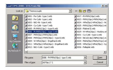
In this example a Pt-PTRh(10%) thermocouple has been loaded into the controller.
