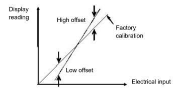
The procedure is exactly the same as shown in the previous section. For the minimum input set the 'CalValue' to the reading required on the controller display as shown in the Low offset in the diagram above.
