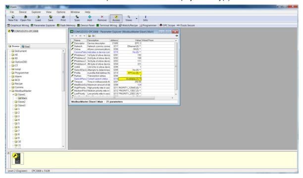
5. We will now configure a second slave but this time using the Fixed comms serial interface making sure that we select "Serial(2)" enumeration for the Network parameter and set the correct Modbus slave address.
