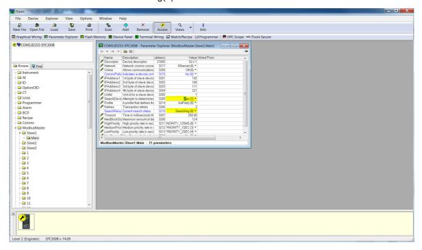
4. If the Modbus slave is online then the search result will be "Available(1)" otherwise the result will be "Unreachable(3). If it is a Eurotherm instrument with a supported profile, the "Profile" parameter will display the Modbus slave's profile otherwise it will display "3rdParty(0)".
