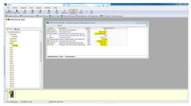
5. For a third party slave (unsupported profile), select "UserDefined" from the Parameter List drop-down and configure the register address, function code, the data type and priority of data read/write.
