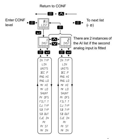
The parameters in the following list are identical for both 1 and 2.
