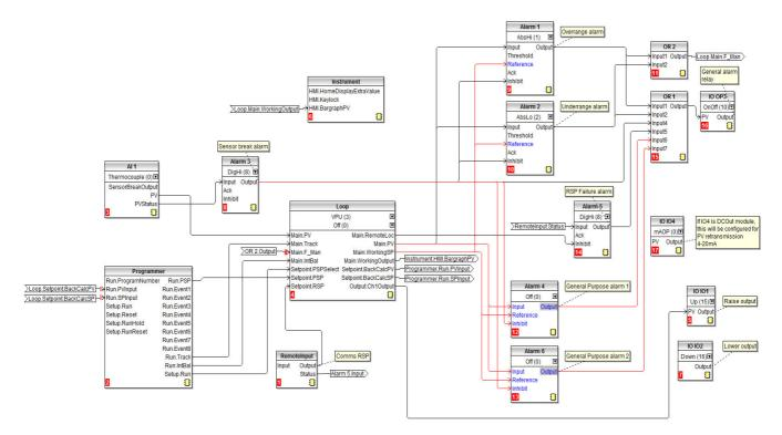
This is the same as a heat only controller except that IO1 is configured for valve raise (Up). This means that IO2 is automatically configured for valve lower (Down) and cannot be wired to any other source. It does not, therefore, need to be shown wired.
