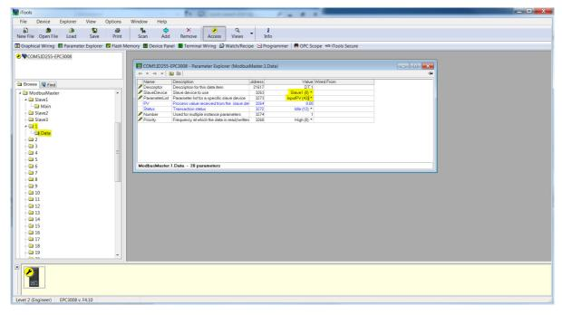
3. To configure a write for a known profile, select parameter to write from the Parameter List drop-down box.
