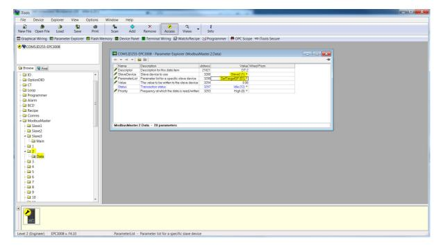
4. For a parameter that is not on the Parameter List. The data configuration has to be done manually. Select "UserDefined" from the Parameter List and configure the register address, function code, the data type and priority of data read/write.
