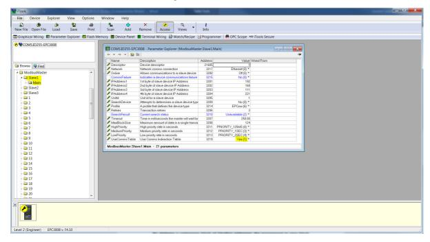
2. In Operator mode, the CommsTab Function Block should now show every configured Modbus Master data. The user can then change Native, ReadOnly and Minutes parameters from default to configure how the data is presented from the Modbus indirection table.
