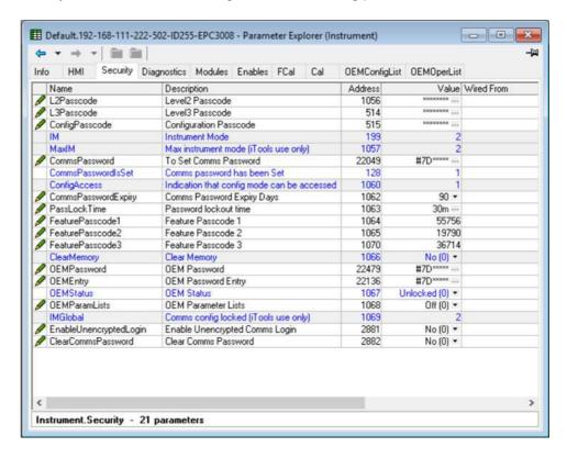
To change the Comms Config password, click on the ellipsis in the value cell on the password dialog window and enter a new value.
