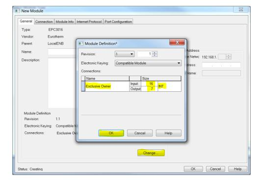
31. On the "New Module" window, configure the IP address of the EPC3000 EtherNet/IP adapter. Enter a descriptive name and then click "OK" button.
