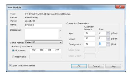
23. Configure connection properties of the newly created module by right-clicking it and selecting "Properties".
