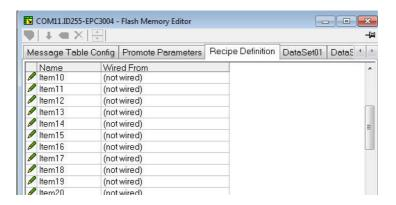
The Recipe Definition table contains a set of 40 parameters. Not all 40 parameters need to be wired.
