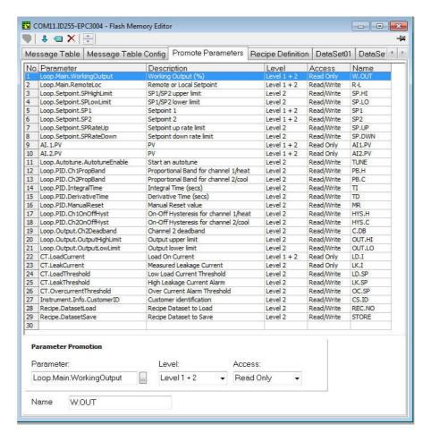
The list shows the parameters which are available in Levels 1 & 2, Level 2 only and whether they are Read Only or Read/Write.
