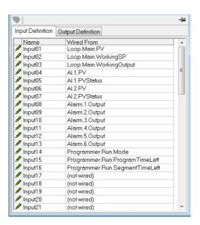
By default, the Input and Output Definition tables are configured with the most frequently used parameters.
