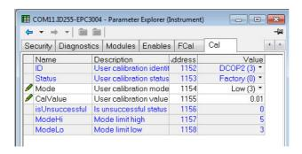
Read the DC output on the meter. For a voltage output, this should read 2.00 volts. (For a mA output this should read 4.00mA). If the voltage reading is 1.90V, enter this value, into the C.VAL parameter as shown below.
