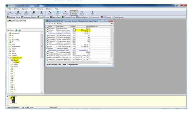
2. Configure the slave's IP Address and unit ID.
