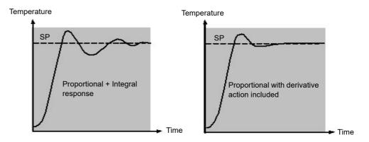
The derivative modifies the output to reduce the rate of change of the difference. It reacts to changes in the PV by changing the output to remove the transient. Increasing the derivative time will reduce the settling time of the loop after a transient change.
