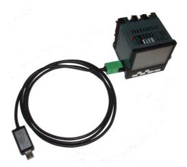
**Note:** In some cases it may be preferable to have the configuration clip connected but not power the instrument from the USB port. For example, when the controller is powered by the standard Low Voltage (24Vdc) or Mains (110Vac -240Vac) and iTools is connected to monitor, configure or clone it. The power can be disconnected by removing Pins 1 & 5 in the following diagram.
