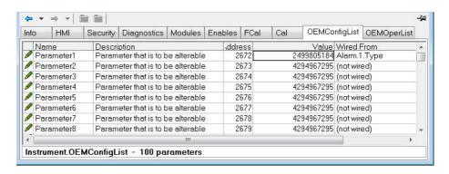
The view shows the first 8 parameters of which Parameter 1 has been populated with a configuration parameter (Alarm 1 Type). Examples of configuration parameters include Alarm Types, Input Types, Range Hi/Lo, Modules Expected, etc.
