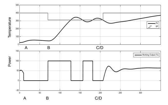
The second example shows Heat/Cool Autotune with 'Standard' Ch2 tune type.
