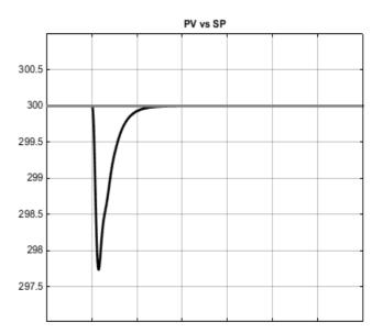
Here, it can be seen that enabling power feedforward has greatly reduced the magnitude of the process disturbance. However, the smaller disturbance persists for a longer period of time.
