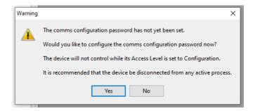
Selecting 'Yes' will automatically launch the iDevPWSetup tool.
