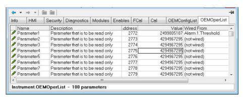
The example shows the first 8 of 100 parameters of which the first has been selected as 'Alarm 1 Threshold'. This parameter is to be read only when OEM Security is enabled and the controller is in Operator access level.
