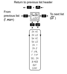
From this list you can configure the switchover function block. This is only appears if the function has been enabled.
