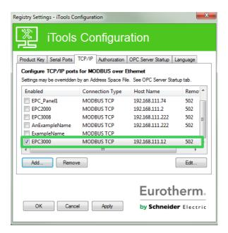
iTools is now ready to communicate with an instrument at the Host Name/IP Address configured.
