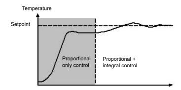
The units for integral are measured in time. The longer the integral time constant, the more slowly the output is shifted and results in a sluggish response. Too small an integral time will cause the process to overshoot and even oscillate. The integral action may be disabled by setting its value to Off(0), in which case manual reset will be made available.
