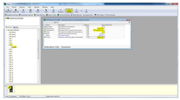
3. To send a write request, set the "Send" parameter. The Status will go to "Pending(13)" briefly before going to "Success" when the parameter has been written. If the write has failed then the Status will show the reason for the failure.
