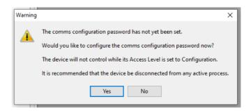
informing the user that they need to configure the Comms Configuration password before being able to proceed. Selecting 'Yes' will automatically launch the iDevPWSetup tool.
