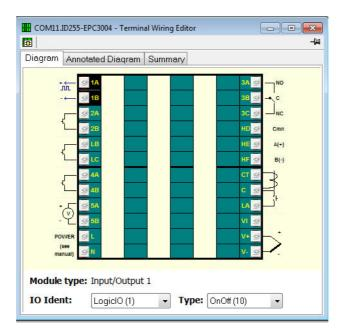
From this view click on a set of terminals representing an IO module. In the 'IO Ident' drop down select an IO type. The diagram of the type of IO will be shown against the chosen terminal set.
