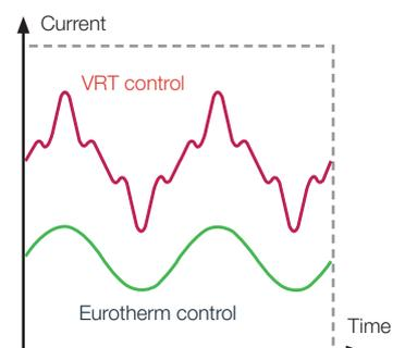
VRTs waste energy by drawing more power from the supply than is required by the heater due to harmonic generation at most setpoint levels.
