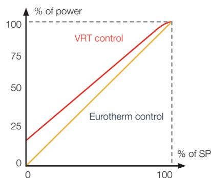
Eurotherm digital thyristor power control helps to provide linear control across the entire output % range, whereas the VRTs cause unstable control at low setpoints.
