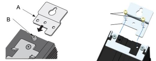
For Bulkhead mounting, fit the upper bracket 'A' to the rear of the unit by removing screw 'B' and associated shakeproof washer, offering the bracket up to the unit, and then securing it using screw 'B' ensuring that the bracket is correctly oriented (as shown) and that the shakeproof washer is fitted between the screw head and the bracket.
