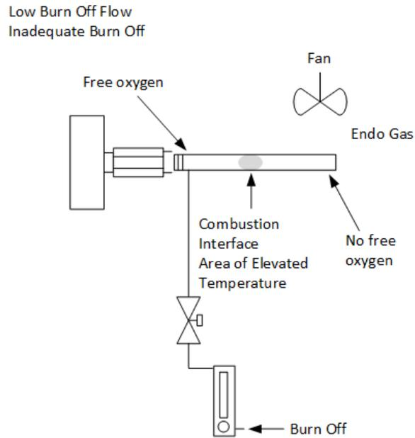
Figure 4 Inadequate Burn Off
