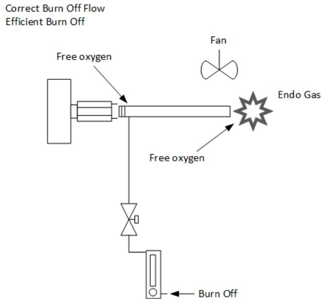
Figure 5 Efficient Burn Off
