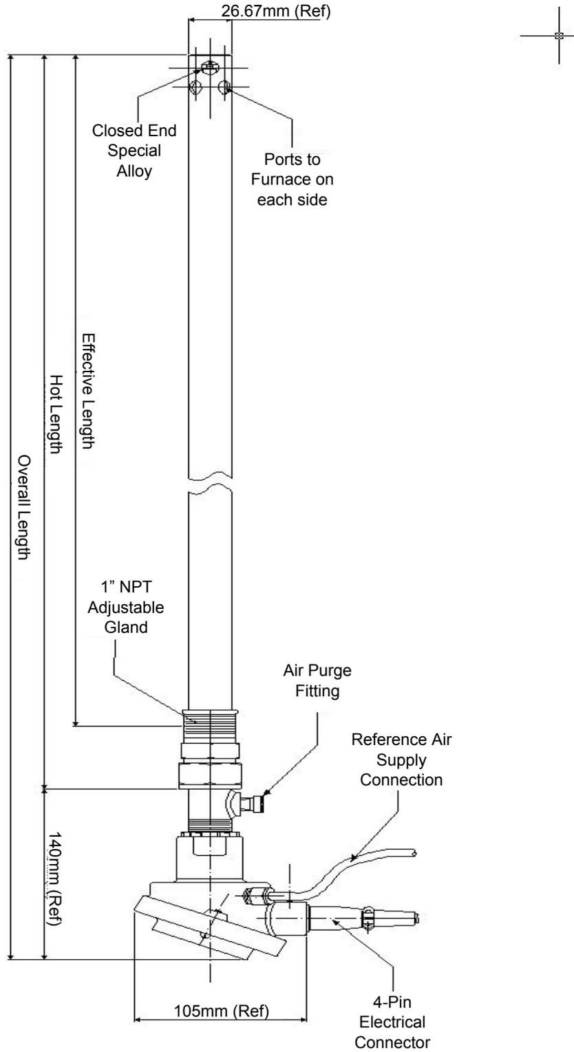
Figure 6 Probe Dimensions
