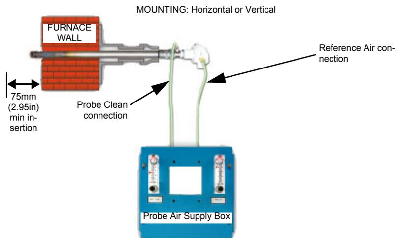
Figure 2 Probe Installation
