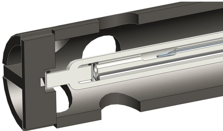
Figure 1 Carbon Probe Cross Sectional View
