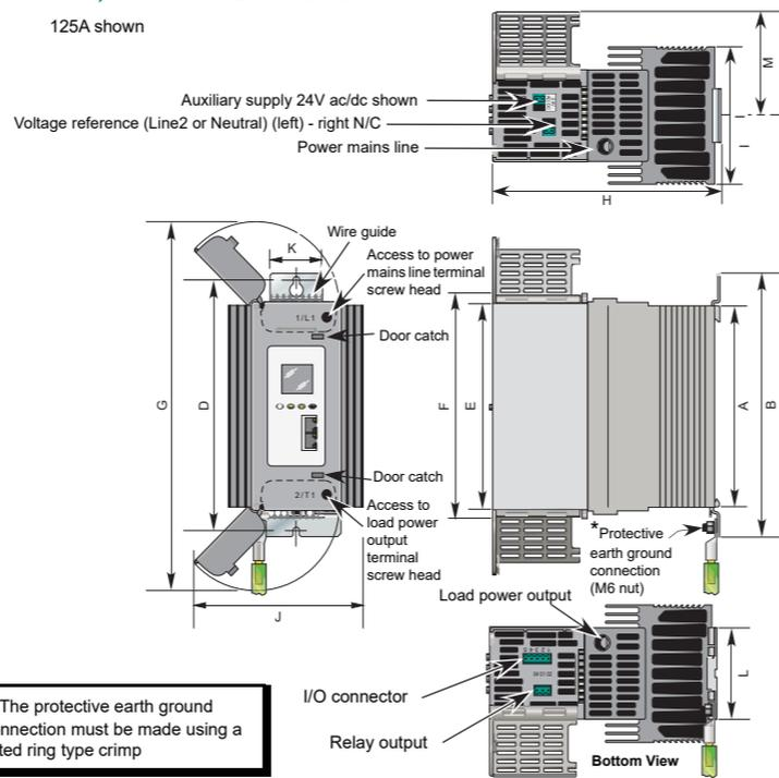
\* The protective earth ground connection must be made using a listed ring type crimp
