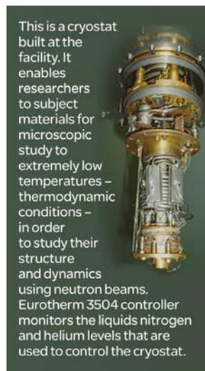
This is a cryostat built at the facility. It enables researchers to subject materials for microscopic study to extremely low temperatures – thermodynamic conditions – in order to study their structure and dynamics using neutron beams. Eurotherm 3504 controller monitors the liquids nitrogen and helium levels that are used to control the cryostat.
