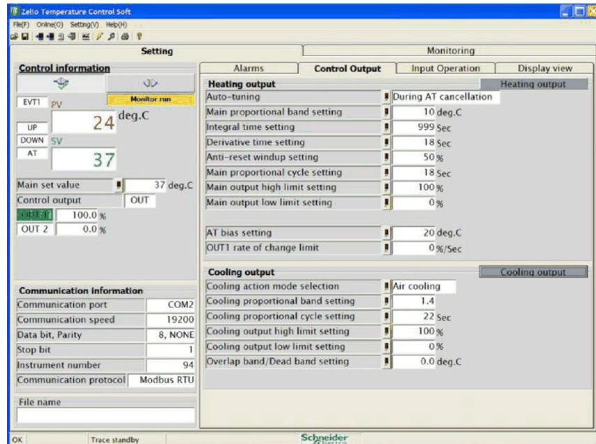
The Control information indicates information about PV, SV, control status, alarm status, monitoring status, and so on. You can set all the parameters on the individual function tab.
