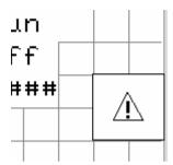
This is a touch button which displays a message page with one or two alarm messages shown. If there are more alarms up/down buttons allow all the active alarms to be viewed.
