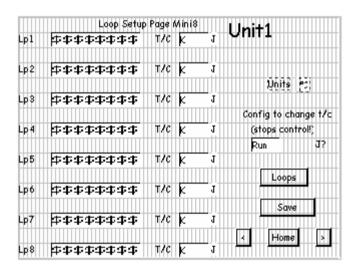
Use the Run/Config button to enter configuration mode.
