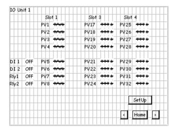
The CT3 module in slot 2 does not have the normal PV values.
