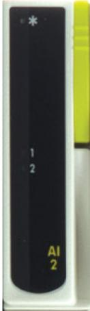
This analog input module is used to monitor analogue signals from a wide range of plant sensors. The mA and TC inputs each require the appropriate terminal unit. The second channel of the AI2 has a special high impedance range for use with zirconia probe inputs for oxygen measurement.
