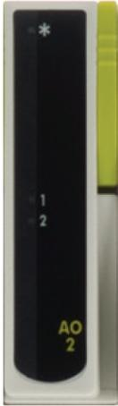
This analog output module provides two isolated analog output channels. Each output can be independently configured for current or voltage.
