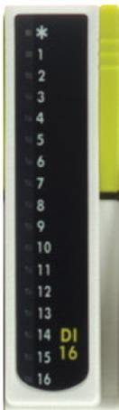
This digital input module accepts sixteen inputs and can be wired either for voltage input or for contact closure.
