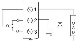
Use a diode with a reverse breakdown voltage two to three times the circuit voltage and forward current at least as large as the load current.
