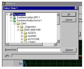
To read the actual value (PV), scroll and expand the 2604 folder (ID001.2604-V300) to LP1\_VIEW/Main and select PV. The folder hierarchy shown differs depending on the Series 2000 instrument connected. Press Ok and continue selecting the items for the number selected. Once complete, the value of the selected items begins to scroll across the chart.
