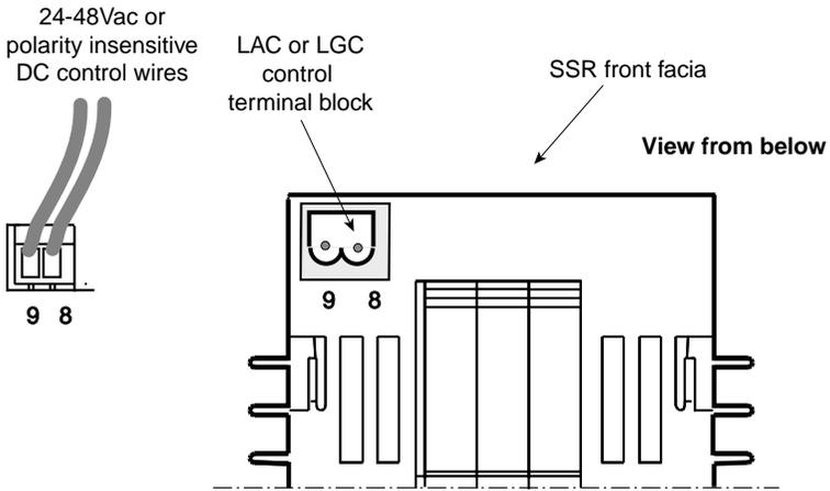
Figure 3-3 Control terminal block for LGC and LAC codes
