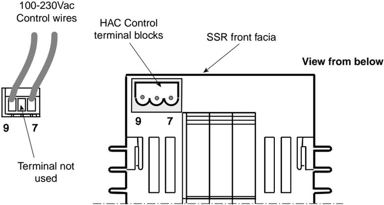
Figure 3-4 Control terminal block for HAC code
