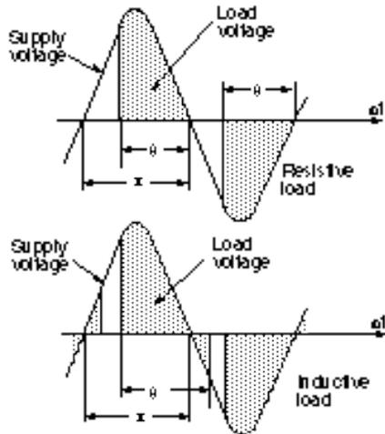
Load voltage in 'phase angle' firing mode
