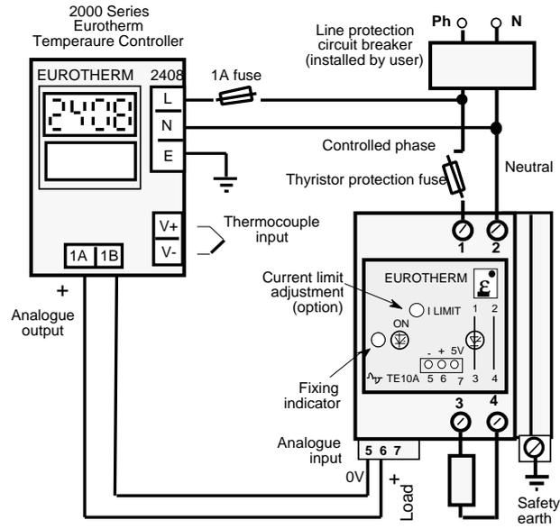
TE10A wiring example (230V supply, input 0 to 10V)
