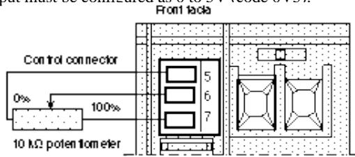
External potentiometer wiring example (view from below)
