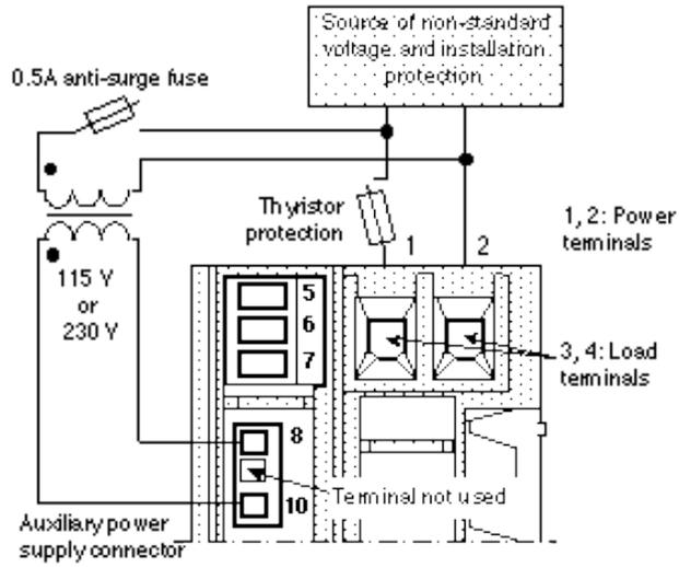
Example of auxiliary power supply wiring with non-standard mains.
