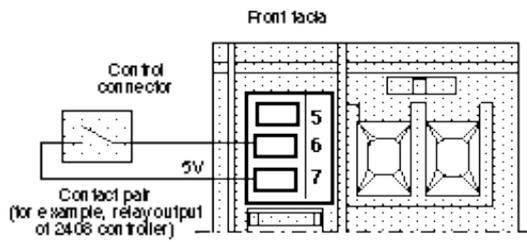
Control contact wiring example (view from below)
