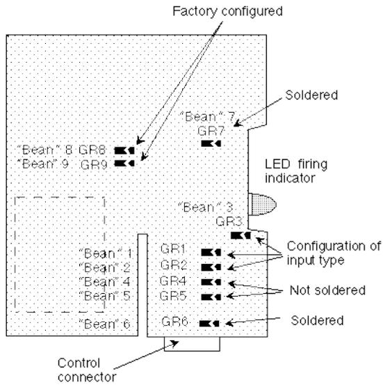
Layout of "Coffee beans" on circuit board (solder side view)
