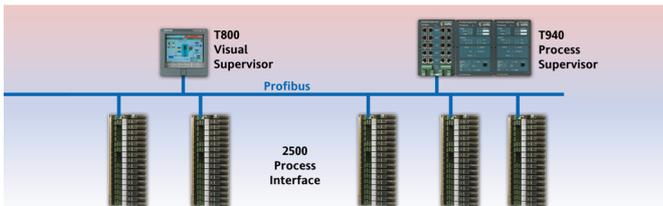
Process Supervisor is designed to use Eurotherm's 2500 for its distributed I/O system. It can also communicate with any third party device that supports Profibus DP or Modbus RTU protocol.
