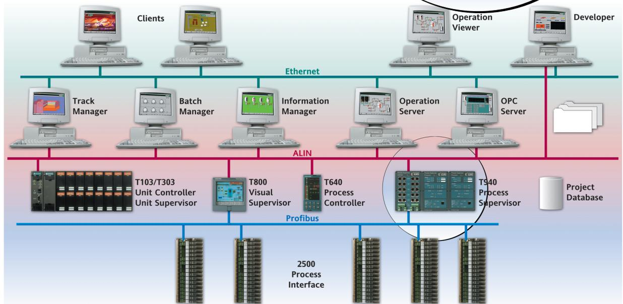
The Process Supervisor is a powerful and configurable strategy engine capable of performing both continuous and sequential control. It has evolved from the successful T103/T102/T100 Unit Controllers and is designed for large applications.
