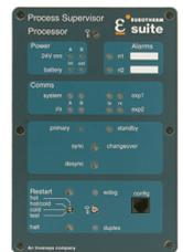
Processor modules can be supplied by two external 24V-power supplies to ensure operation in the event of power failure. The LEDs on the front panel of the Processor Modules provide comprehensive status indication, allowing for rapid verification and diagnostics.
