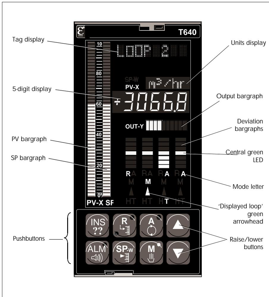
Figure 4-1 T640 front panel — the operator interface
