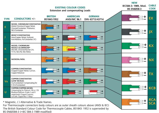
Additional identification as to whether a thermocouple cable type is extension or compensating is indicated in the example which follows; however, please note that a letter A or B after the C for Compensating refers to the Cable Temperature Range in accordance with the Table of Tolerance Values set out with this standard.
