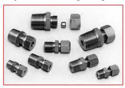
The Eurotherm range of adjustable mounting fittings (compression couplings) allow the positioning of probes to achieve the desired immersion depth in the process. They are also used to couple the probe with a thermowell or thermopocket. Brass and stainless steel versions are offered.
