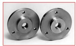
The Eurotherm flange plates enable the mounting of probes with compression fittings. Available in stainless steel and brass, flange plates are particularly recommended for mounting probes in process ovens, kilns, heating and ventilation ducts.
