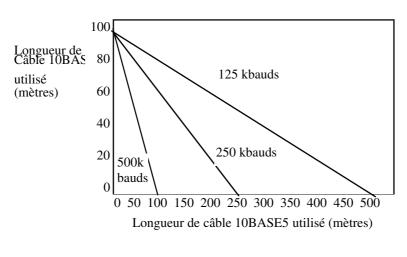
$$\begin{array}{lll} L_{thick} + 5 \text{ x } L_{thin} = 500 & & \text{à } 125 \text{ kbauds} \\ L_{thick} + 2.5 \text{ x } L_{thin} = 250 & & \text{à } 250 \text{ kbauds} \\ L_{thick} + L_{thin} = 100 & & \text{à } 500 \text{ kbauds} \end{array}$$
