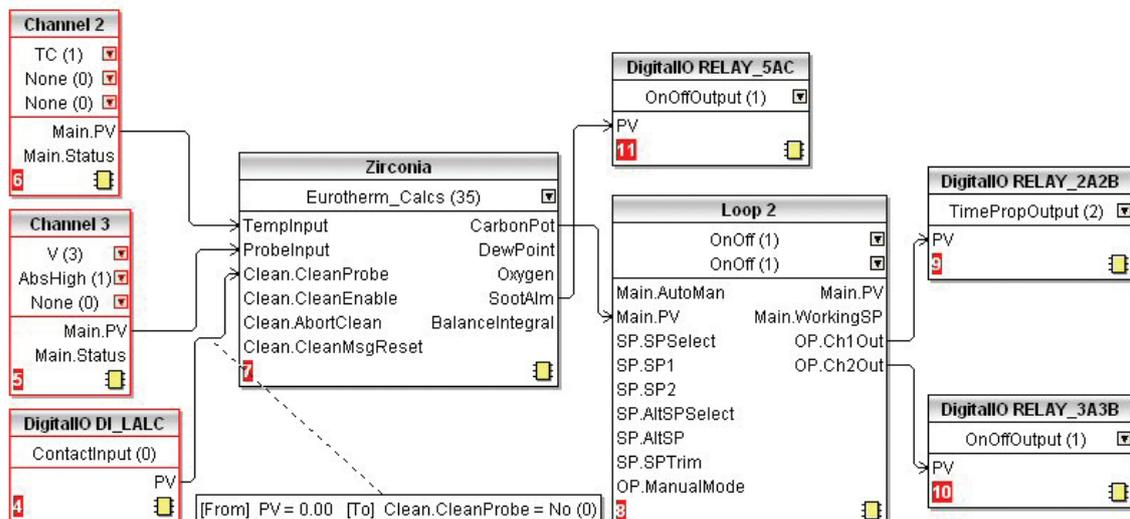
Graphical View of 'Soft' Wiring using iTools
