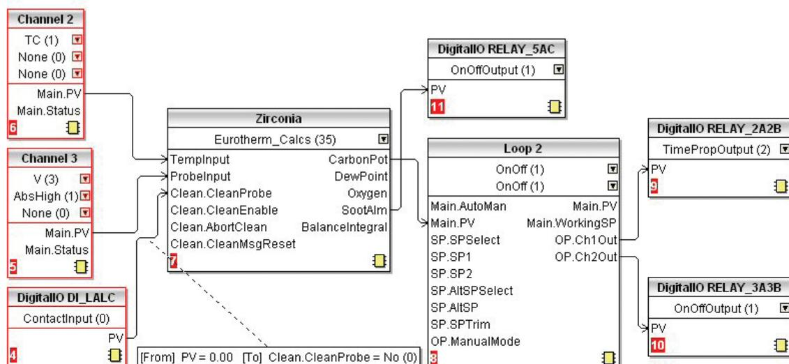
Graphical View of 'Soft' Wiring using iTools
