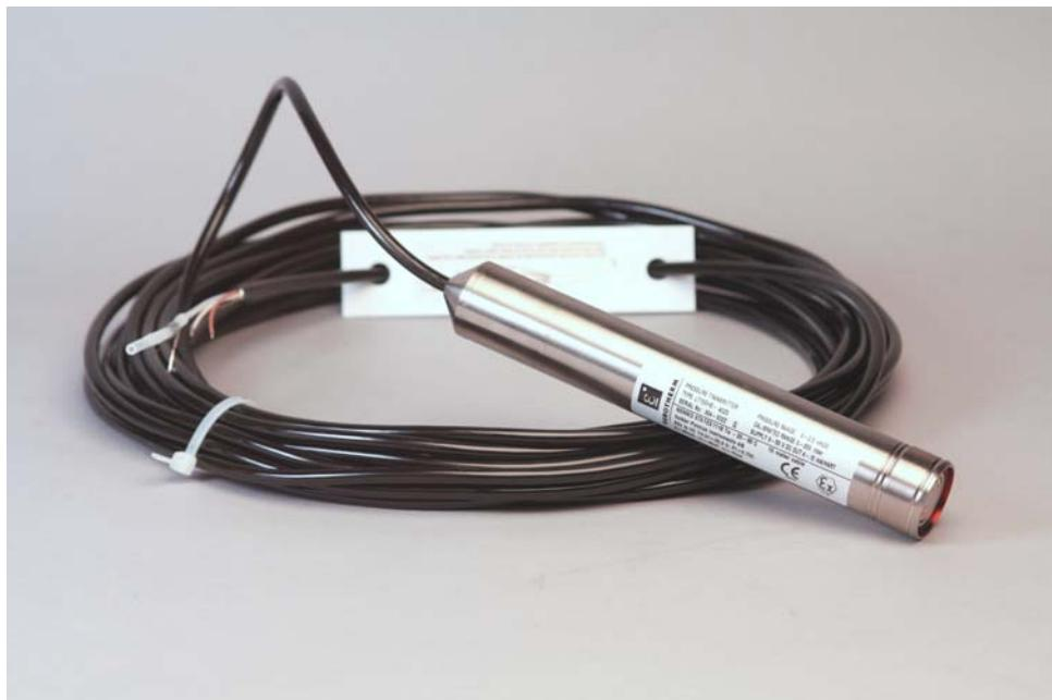
**Level transmitter with submersible probe in stainless steel for applications where pressure connection in the bottom is not possible or desirable. E.g. pump pits, reservoirs or plastic tanks.**
