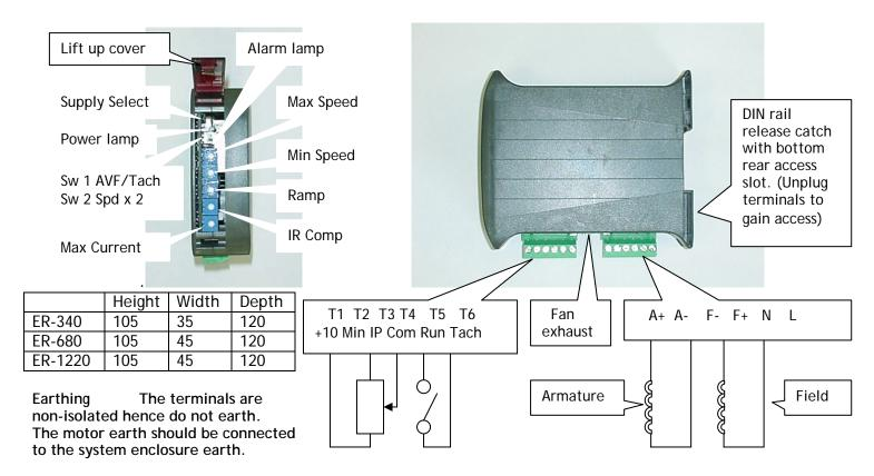
WARNING. This product is non-isolated hence all terminals are at dangerous line potential. Ensure connected items (e.g. speed pot, tach etc.) are not earthed and have sufficient dielectric strength to avoid breakdown.
