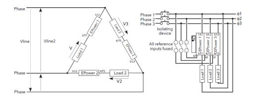
However, the above requirements are not needed to control certain types of application, such as SiC element based tin bath roof heating systems in the glass industry. This was one of the most important types of application considered by Eurotherm during the design of the EPower range in terms of possible efficiency improvements, and it resulted in the recommendation of using two leg burst firing control either in star or delta configuration, as in Figure 3 and Figure 4.
