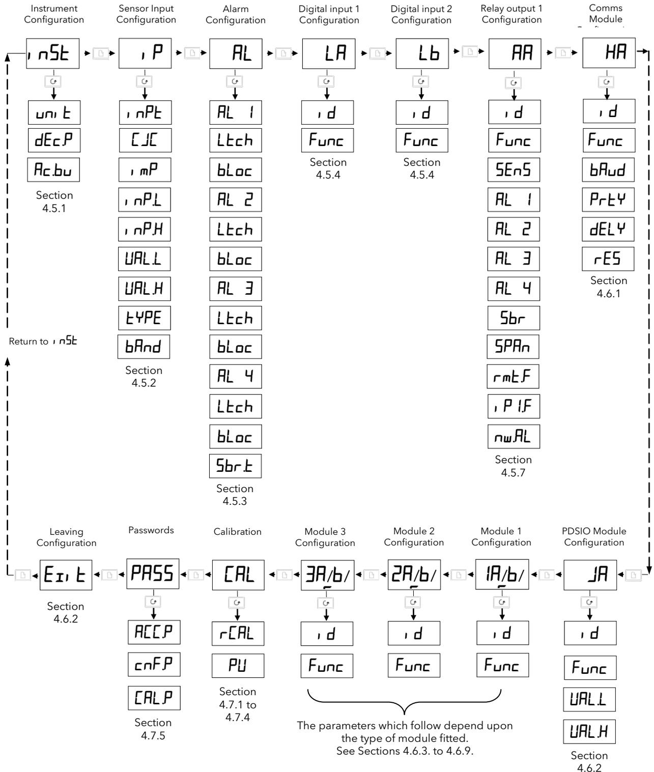
Figure 4-3: Navigation Diagram
