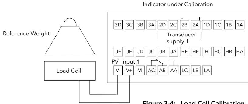
This diagram shows connections to input 1/main input
