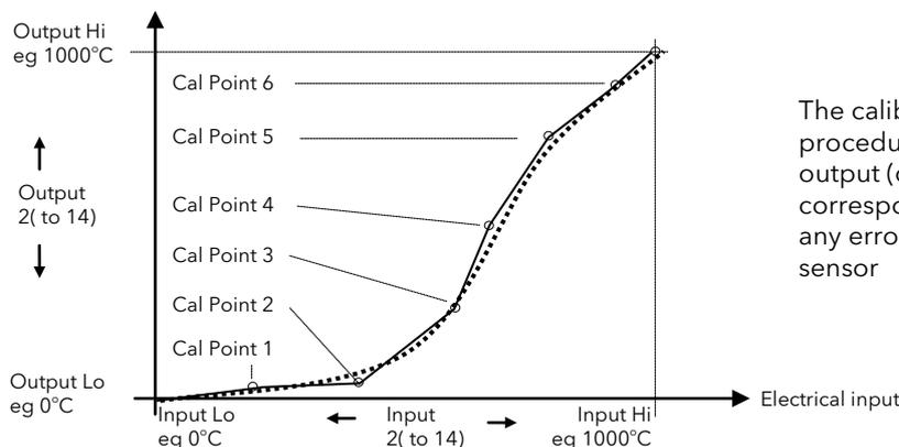
The calibration of the sensor uses the same procedure as described above. Adjust the output (displayed) value against the corresponding input value to compensate for any errors in the standard linearisation of the sensor
