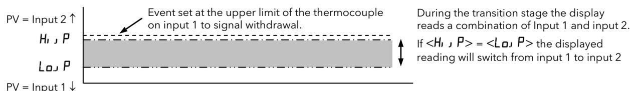
Figure 4-8: Input 1/Input 2 Transition
