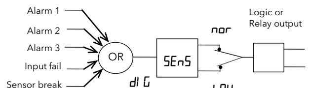
Any combination of alarms can operate the relay or logic output. The diagram shows typical alarms
