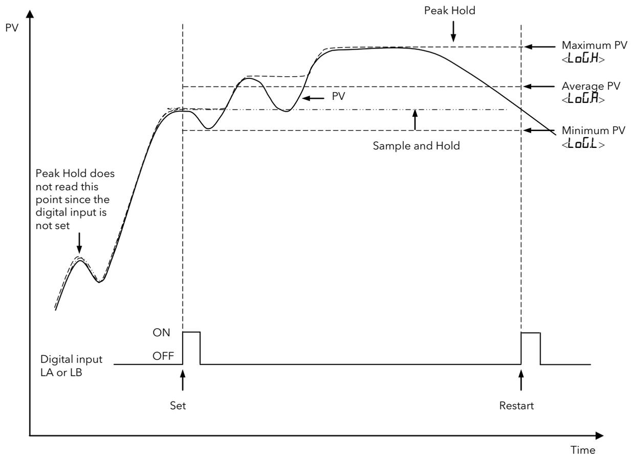
Figure 4-5: Action of Sample and Hold and Peak Hold
