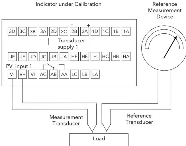
This diagram shows connections to Input 1/main input
