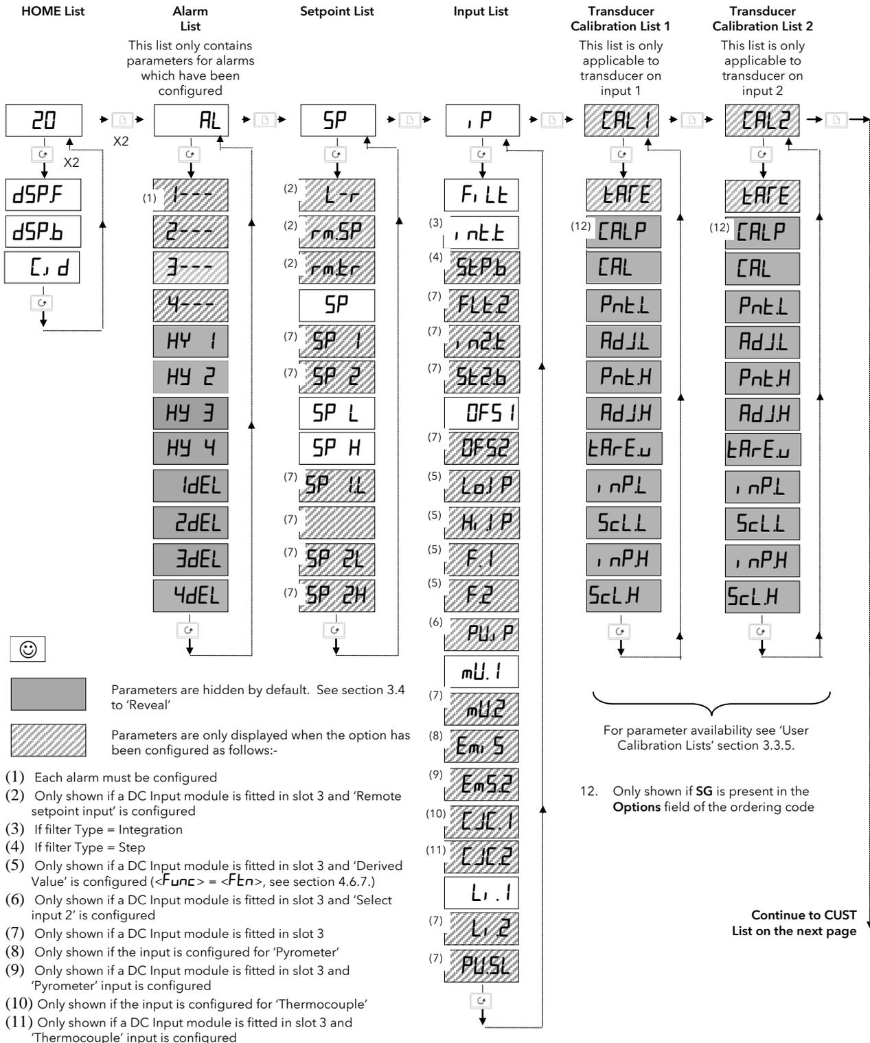
Figure 3-1: Navigation Diagram
