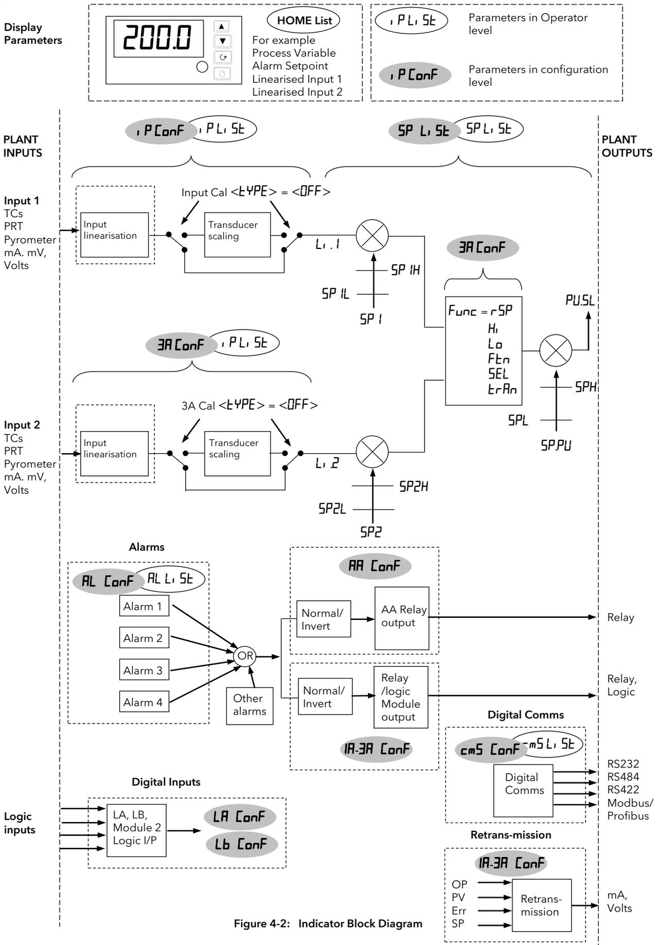
Figure 4-2: Indicator Block Diagram
