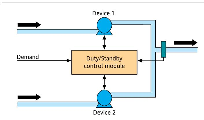
Some of the functions provided by the Duty/Standby control module are:
