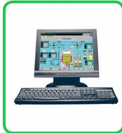
**Historian – Information Manager:** combines the power and flexibility of a relational database with the speed and compression of a real time historian package. The information manager is up to 300 times faster than a conventional relational database but only uses 2% of the disk space normally required by a conventional relational database.
