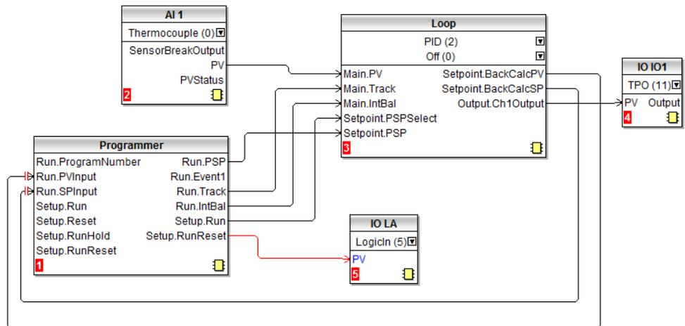
Soft wiring is carried out using iTools and is described in section "Graphical Wiring" on page 80.
