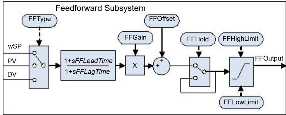
The Loop incorporates a feedforward controller in addition to the normal feedback (PID) controller; it is capable of static or dynamic feedforward compensation. Broadly, there are three common uses for feedforward in these instruments and are described in turn below.
