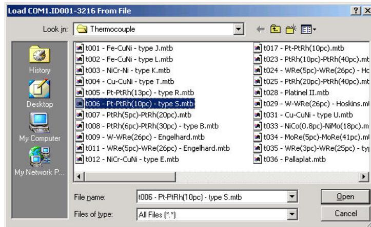
In this example a Pt-PtRh(10%) thermocouple has been loaded into the controller.
