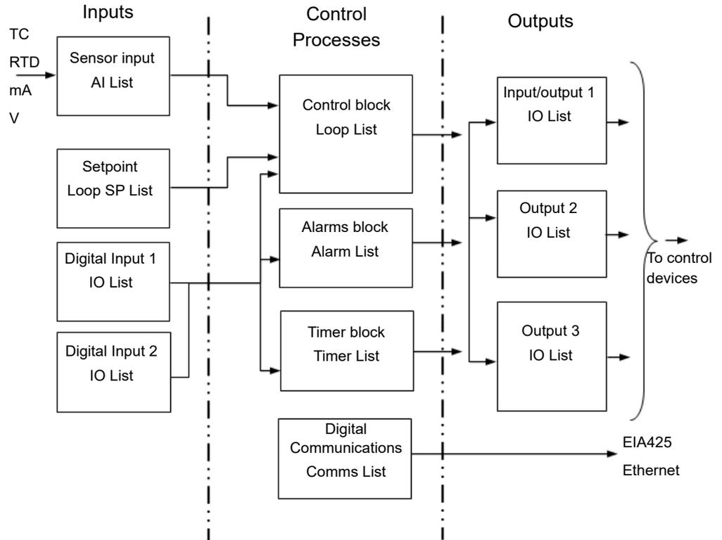
The Temperature (or Process Value, PV) is measured by the sensor and compared with a Setpoint (SP) set by the user.
