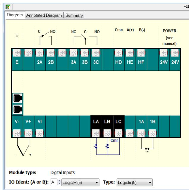
From this view click on a set of terminals representing an IO module. From the 'IO Ident' drop-down, select an IO type. The diagram of the type of IO will be shown against the chosen terminal set.
