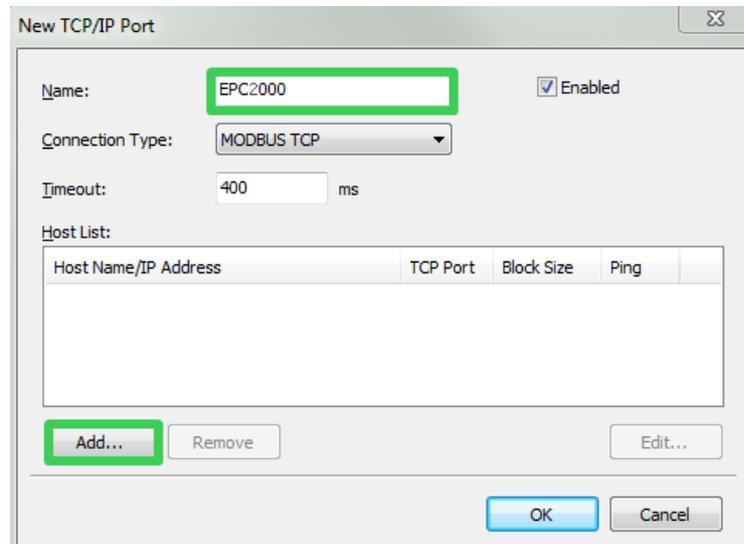
6. The Edit Host panel appears, enter the IP address of the device ensuring that the PC IP address is in the same range as the EPC2000 Programmable Controller then click OK.
