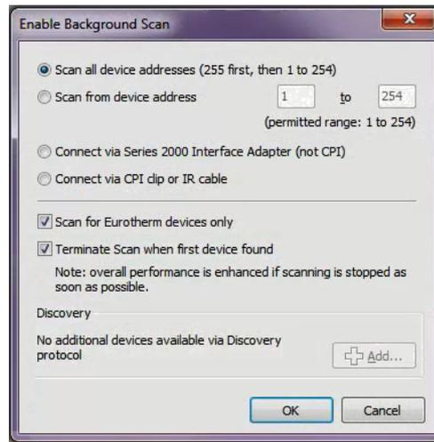
11. If not selected, select Scan all device addresses (255 first, then 1 to 254) option on the Enable background Scan panel, then check the following checkbox options:
