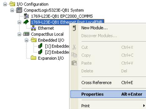
5. In the Module Properties window, configure the IP address and click OK.
