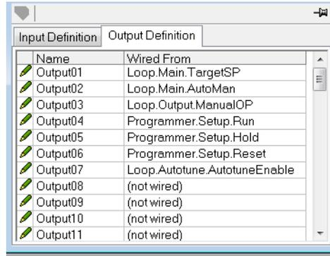
When the definition tables are populated with the variables required, note how many 'wired' entries are included in the input and output areas as this will be needed when setting up the I/O scanner.
