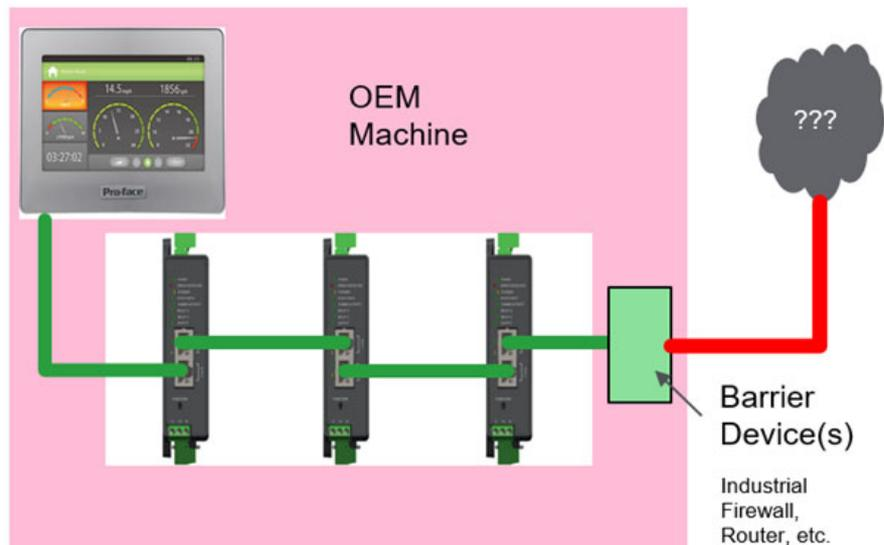
Additionally, it is recommended that the EPC2000 Programmable Controller 'preferred master' parameters are configured with the IP address of the HMI panel to help ensure that the HMI is able to connect to the EPC2000 Programmable Controller even if the other TCP sessions are currently active.
