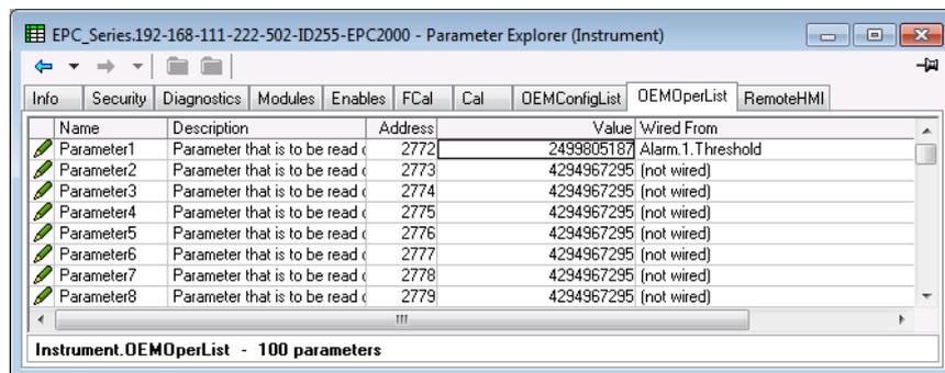
The example shows the first eight of 100 parameters of which the first has been selected as 'Alarm 1 Threshold'. This parameter is to be read only when OEM Security is enabled and the controller is in Operator access level.
