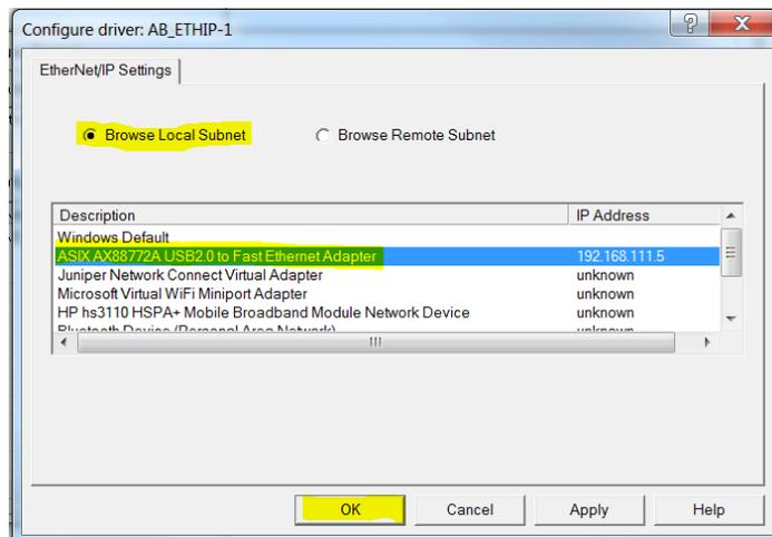
7. PC Serial and EtherNet/IP drivers must now be running. Minimize window.
