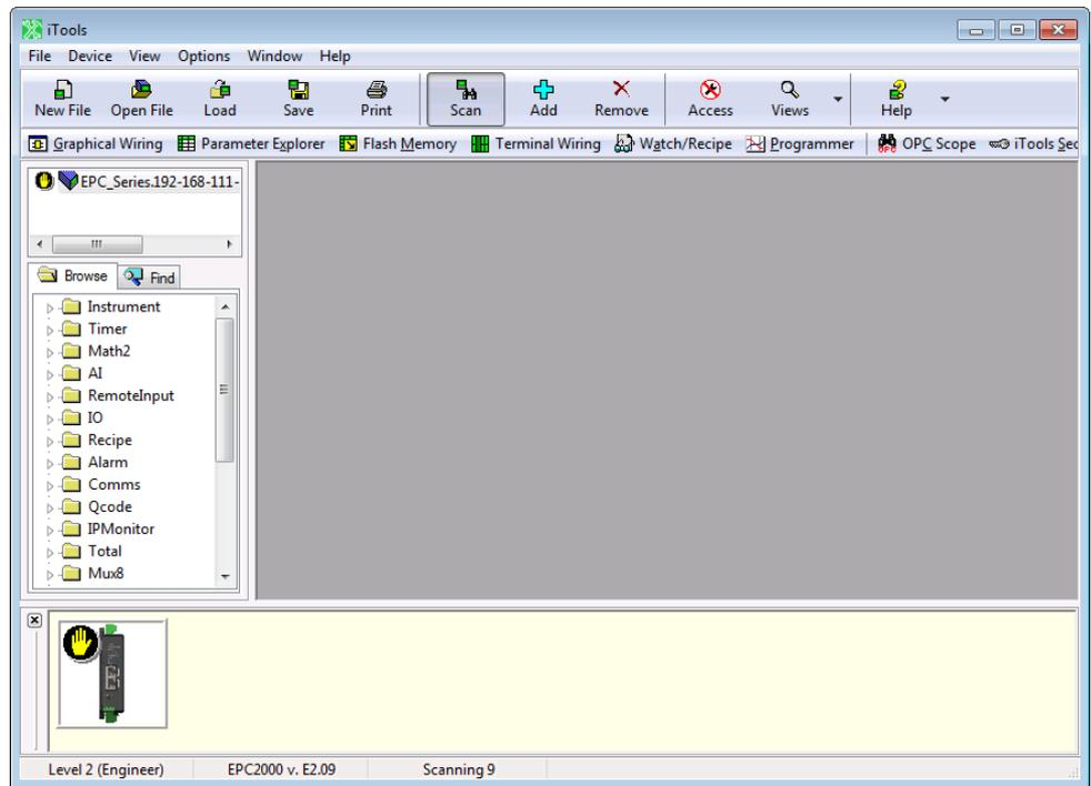
The controller may be configured using the Browser view above. The following pages show a number of examples of how to configure various functions.
