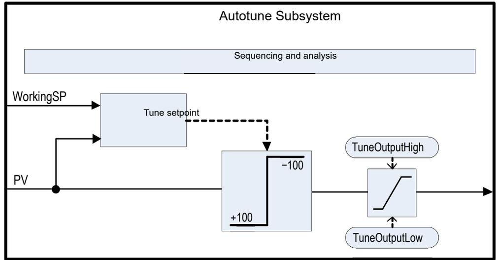
The function block contains sophisticated autotuning algorithms that can tune the controller to the process. They work by performing experiments on the plant, by inducing perturbations, and observing and analysing the response. The autotuning sequence is described in detail below.
