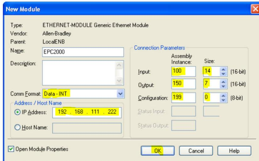
4. Configure connection properties of the newly created module by right-clicking it and selecting "Properties".
