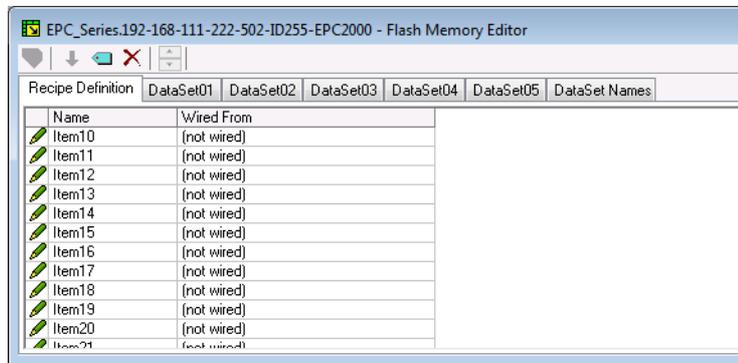
The Recipe Definition table contains a set of 40 parameters. Not all 40 parameters need to be wired.
