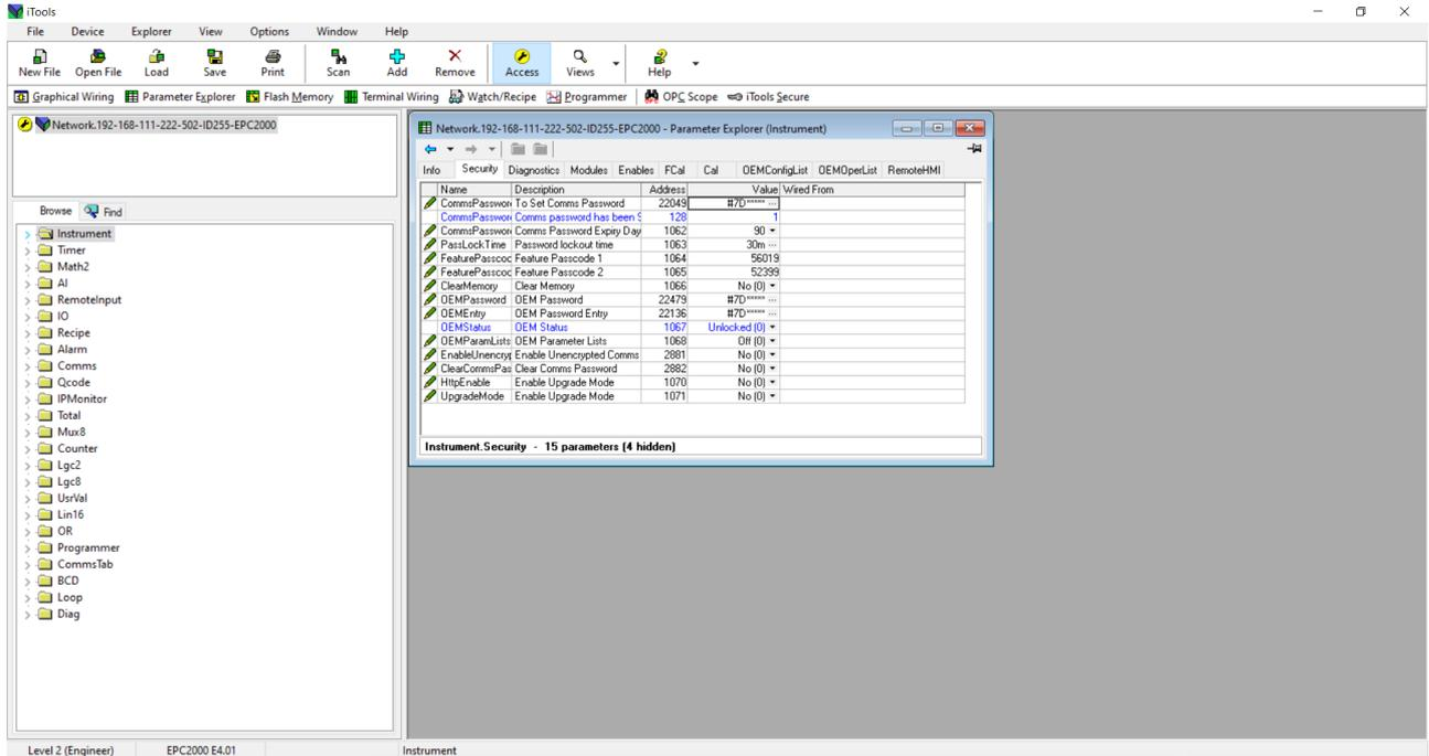
To change the configuration password, click on the ellipsis in the value cell on the password dialog window and enter a new one. The maximum password length is 96 bytes (UTF-8 encoded). The number of characters is therefore dependent upon the character set used. For example:
