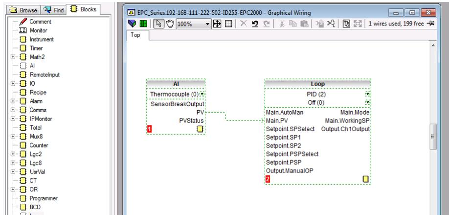
A list of function blocks is shown in the left hand side. Blocks are dragged and dropped from the list into the Graphical Wiring section on the right.
