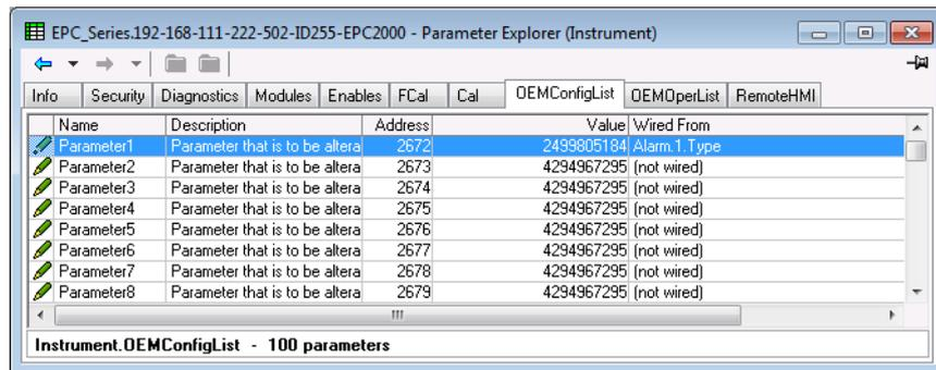
The view shows the first eight parameters of which Parameter 1 has been populated with a configuration parameter (Alarm 1 Type). Examples of configuration parameters include Alarm Types, Input Types, Range Hi/Lo, etc.
