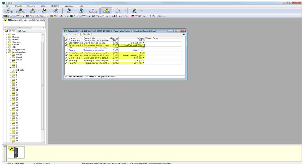
3. For a third party slave (unsupported profile), select “UserDefined” from the Parameter List drop-down and configure the register address, function code, the data type and priority of data read/write.
