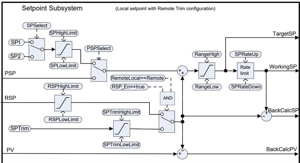
The setpoint subsystem resolves and generates the working setpoint for the control algorithms. The working setpoint can ultimately come from several different sources, programmer, local or remote, have local or remote trims applied, and be limited and rate limited.
