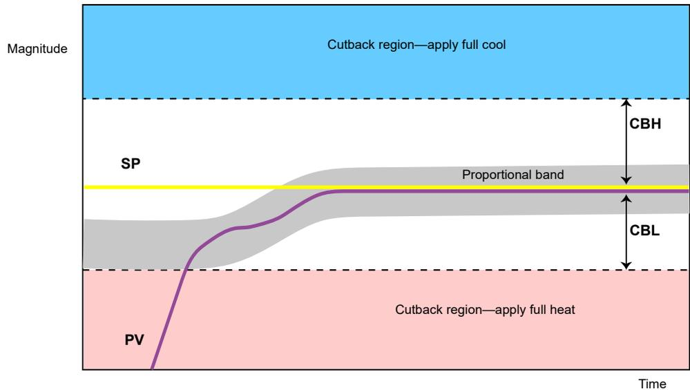
**Note:** Because cutback is a type of non-linear controller, a set of CBH and CBL values that are tuned for one particular operating point may not be satisfactory for another operating point. It is advisable therefore not to try to tune the cutback values tightly, or otherwise to use gain scheduling to schedule different values of CBH and CBL at different operating points. All the PID tuning parameters can be gain scheduled.
