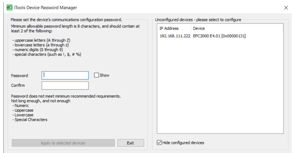
11. Once the password has been set, the EPC2000 Programmable Controller connects with the instrument in configuration mode and the following items appear:
