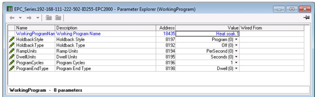
The Working Segment provides read/write access to the segment parameters of the currently running program (which can be the main program or a subroutine resulting from a call segment).
