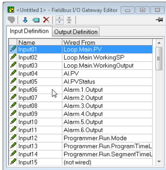
By default, the Input and Output Definition tables are configured with the most frequently used parameters.
