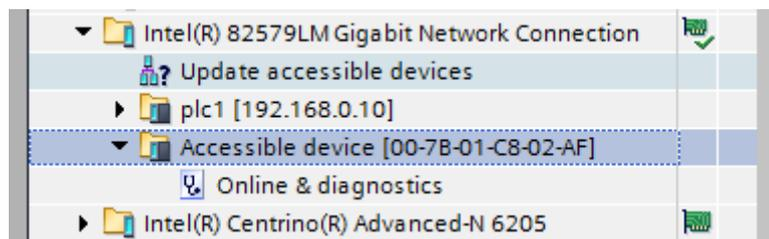
The next step assigns the 'IP Configuration' and the 'Device Name'. This operation can be performed by clicking on the 'Online & diagnostics'.
