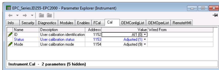
It may be found useful to open the AI function block when carrying out the calibration since the PV can be read directly during the calibration procedure. This also allows the input measurement settling to be viewed during the calibration process.
