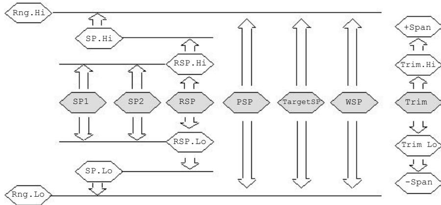
Span is taken to be the value given by Range High Limit - Range Low Limit.
