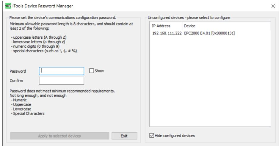
12. Once the password has been set, the EPC2000 Programmable Controller connects with the instrument in configuration mode and the following items appear:
