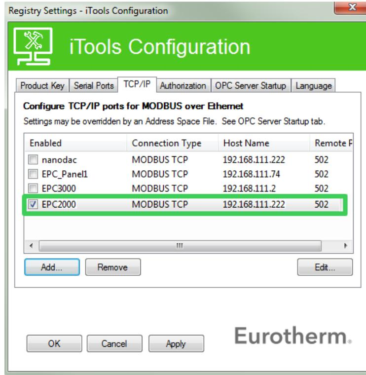
iTools is now ready to communicate with the EPC2000 Programmable Controller at the Host Name/IP Address configured.
