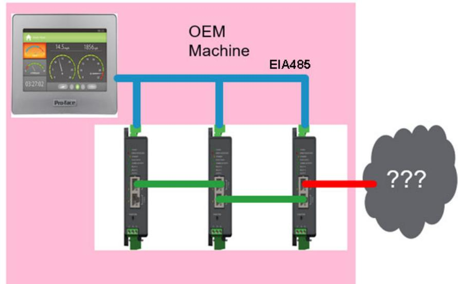
It should be noted that EIA485 communications is given priority over Ethernet communications, however, EIA485 is slow in comparison and therefore consideration should be given to the latency between the EPC2000 Programmable Controller and the HMI via EIA485.
