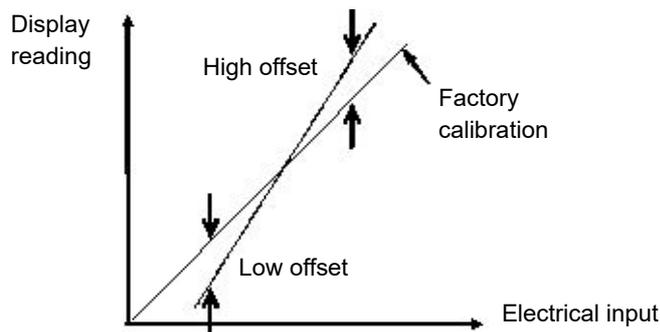
The procedure is exactly the same as shown in the previous section. For the minimum input set the 'CalValue' to the reading required on the controller as shown in the Low offset in the diagram above.
