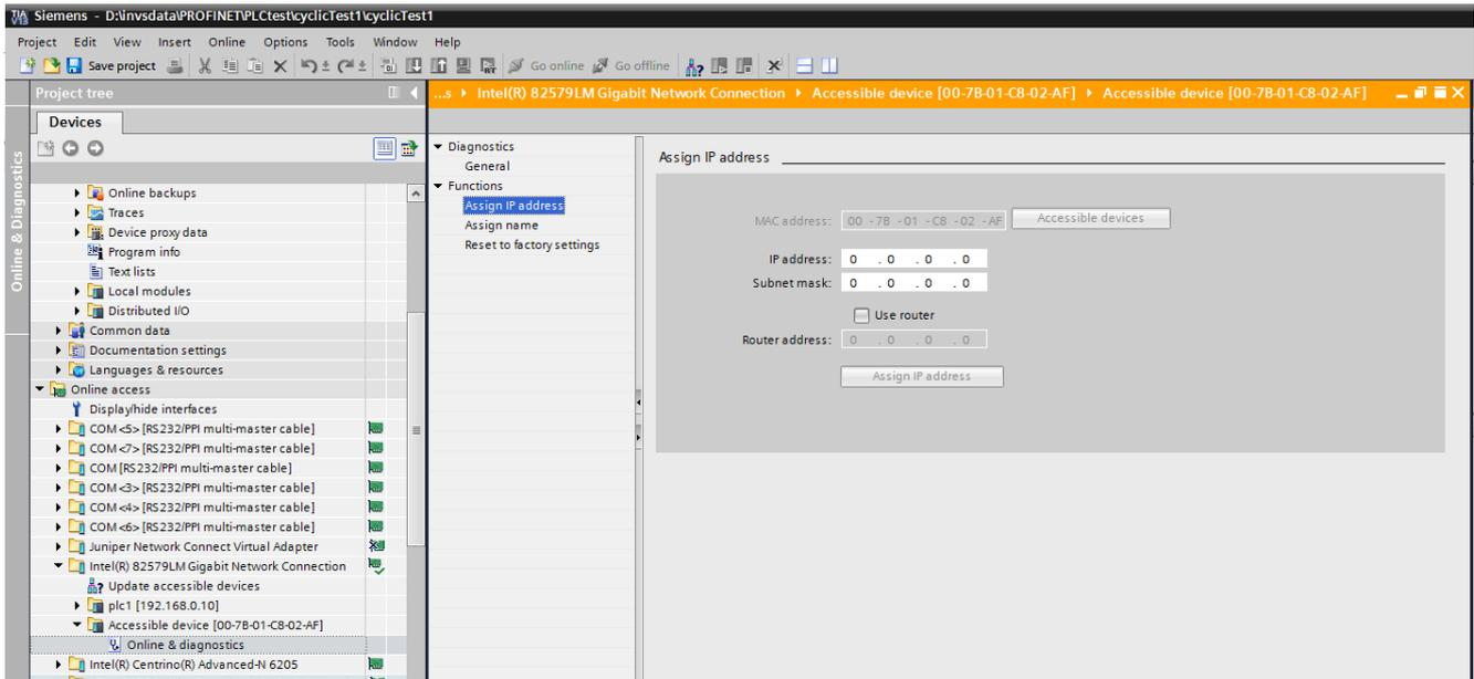
**Note:** The Default Gateway can be changed in the same way (named 'Router address' in this example).
