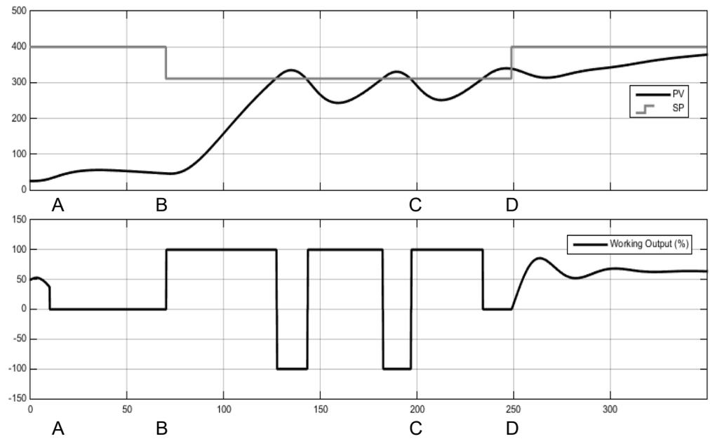
The third shows an example of Heat/Cool Autotune from above with output rate limiting.
