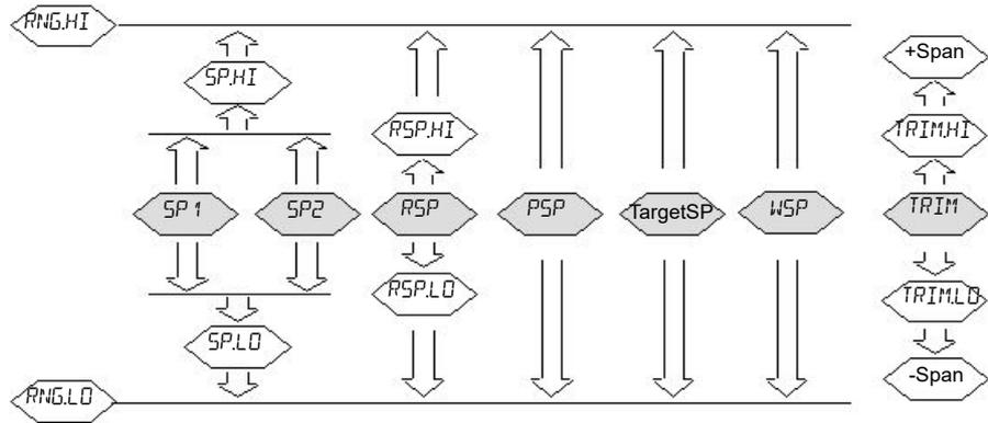
The *Span* is taken to be the value given by  $(RangeHigh - RangeLow)$ .
