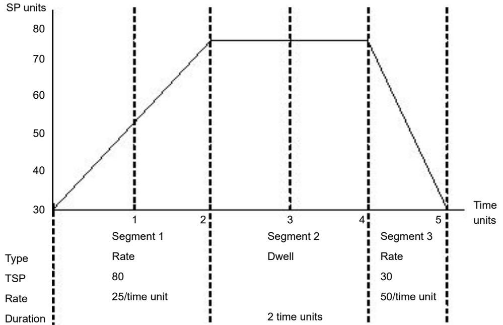
The example above shows a simple three segment program in which the Target Setpoint (TSP) increases at a controlled rate of 25/time unit to a value of 75. It then dwells at that setpoint for two time units before decreasing to 30 at a controlled rate of 50/time unit.
