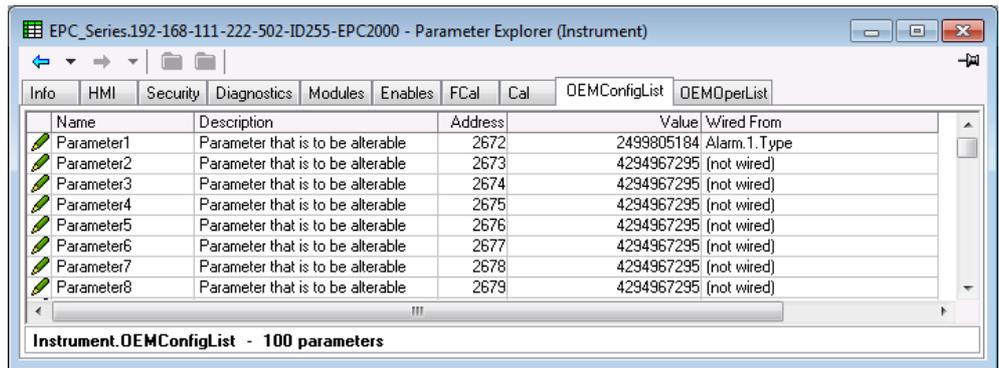
The view shows the first eight parameters of which Parameter 1 has been populated with a configuration parameter (Alarm 1 Type). Examples of configuration parameters include Alarm Types, Input Types, Range Hi/Lo, Modules Expected, etc.
