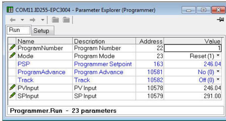
To run a program make sure that the controller is in Operator mode and that the PVInput parameter status is 'Good'. Select the program number of the program to run and select Run(2) from the Mode parameter drop-down enumeration. The program may also be put into Hold or Reset from the mode Parameter.
