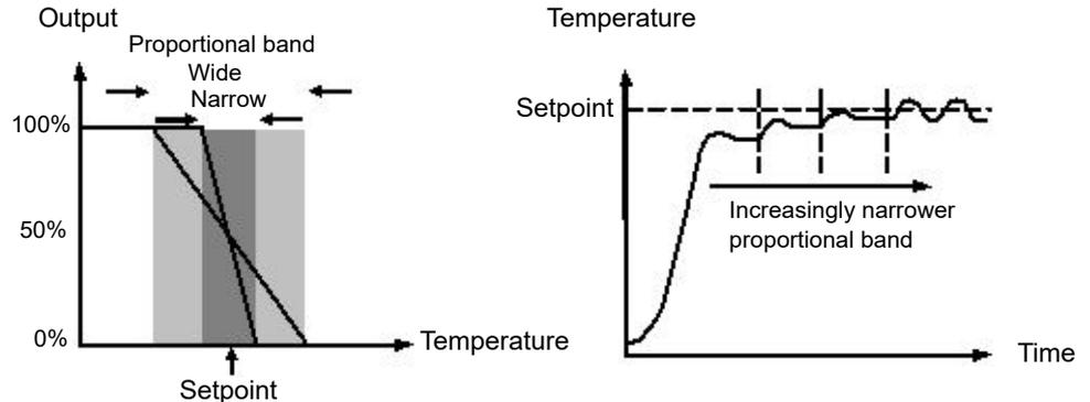
The diagram also shows the effect of narrowing proportional band to the point of oscillation. A wide proportional band results in straight line control but with an appreciable initial error between setpoint and actual temperature. As the band is narrowed the temperature gets closer to setpoint until finally becoming unstable.
