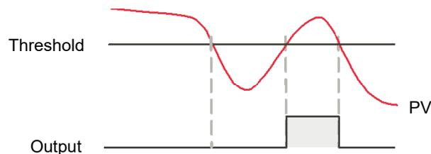
Blocking will be enforced after a power-cycle or after exit from configuration depending upon the latching status of the alarm as follows:
