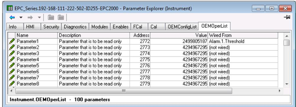
The example shows the first eight of 100 parameters of which the first has been selected as 'Alarm 1 Threshold'. This parameter is to be read only when OEM Security is enabled and the controller is in Operator access level.
