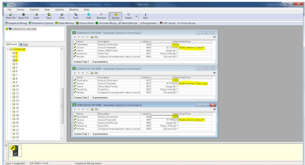
The screenshots below show Modbus Master data auto-configured to appear at the Modbus Indirection table and the values read by a third party Modbus Master from a Eurotherm Modbus Master device:
