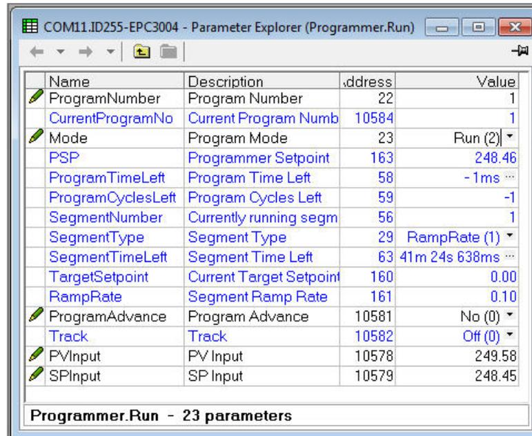
When one of the programs (Program 1 to 10) is run, the program parameters are copied into the working program. The Working Program and Working Segment parameters are then made available for monitoring and/or editing.
