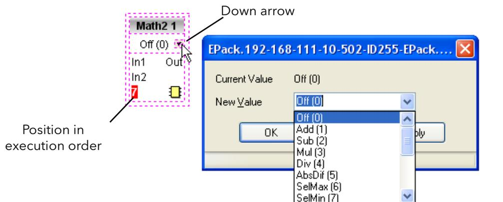
Figure 134 Function block example
