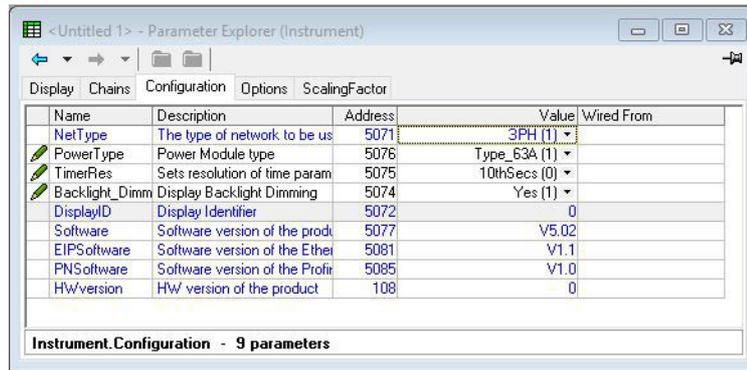
Figure 107 Instrument configuration
