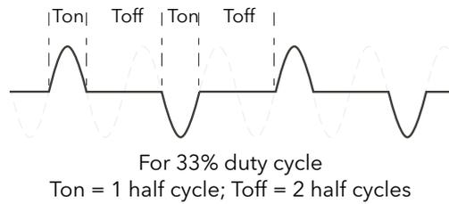
Figure 24 Intelligent half cycle mode: 33% duty cycle
