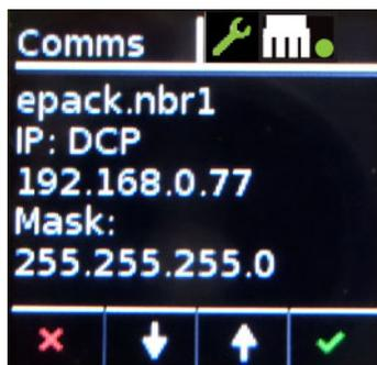
Figure 49 Display of the Device Name on EPack (e.g. “epack.nbr1”).
