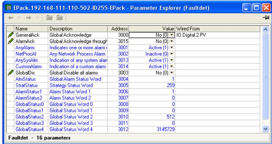
Figure 93 Fault detection menu page
