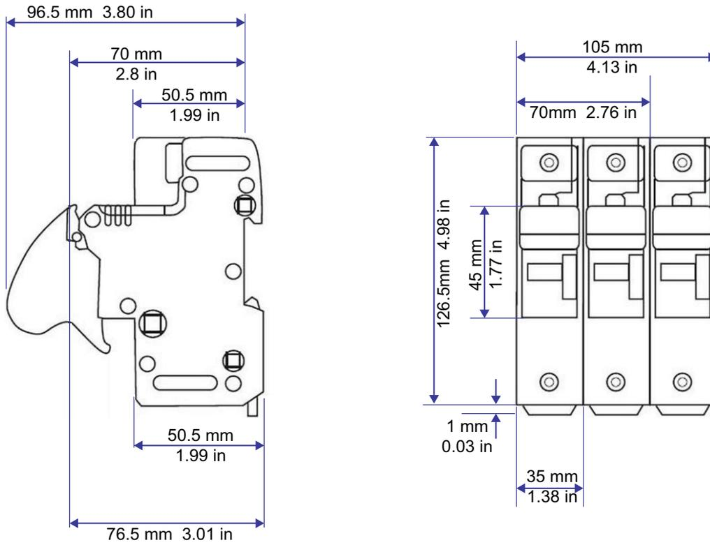
Figure 153 Fuse holder dimensions: US223 (22x58mm)
