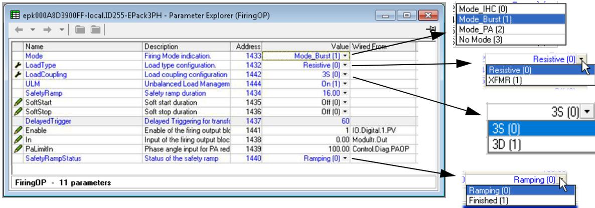
Figure 94 iTools configuration firing output page
