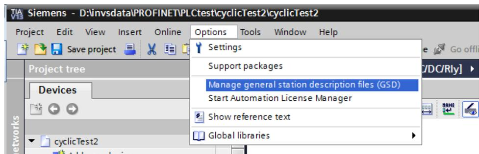
Figure 50 Loading the EPack GSDML file into STEP7
