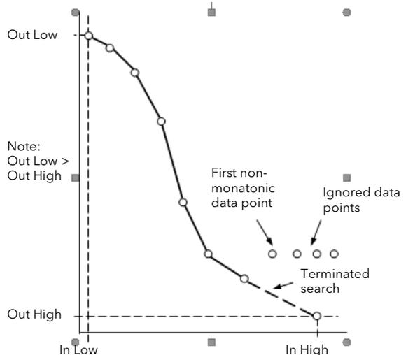
Figure 117 How an Inverted Curve will Terminate its search when it detects non-monotonic data
