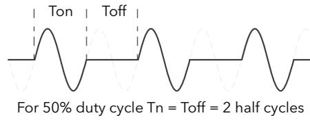
Figure 23 Intelligent half cycle mode: 50% duty cycle
