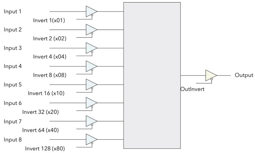
Figure 115 LGC8 Schematic
