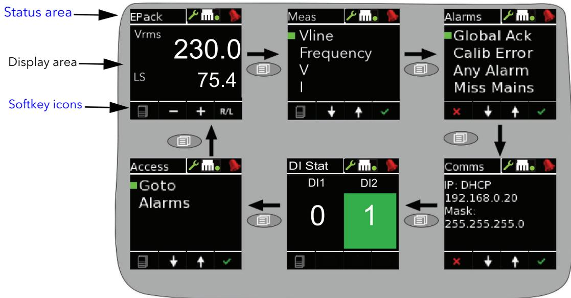
Figure 16 Operator interface
