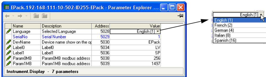
Figure 106 Instrument display configuration page
