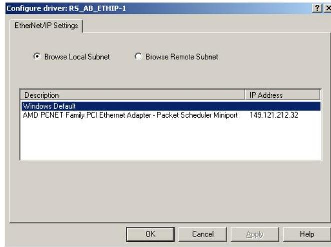
Figure 39 RSLinx Classic configure driver Ethernet/IP settings
