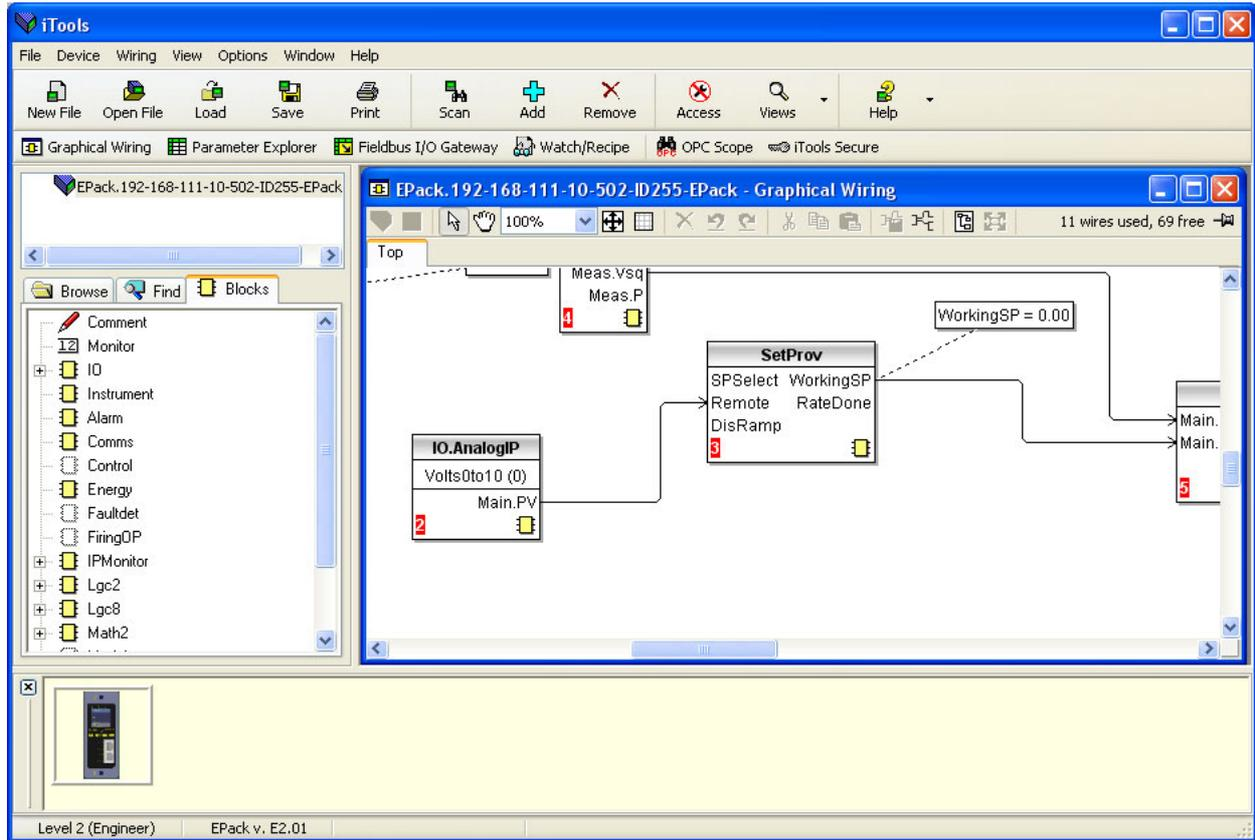
Figure 133 Graphical wiring Editor
