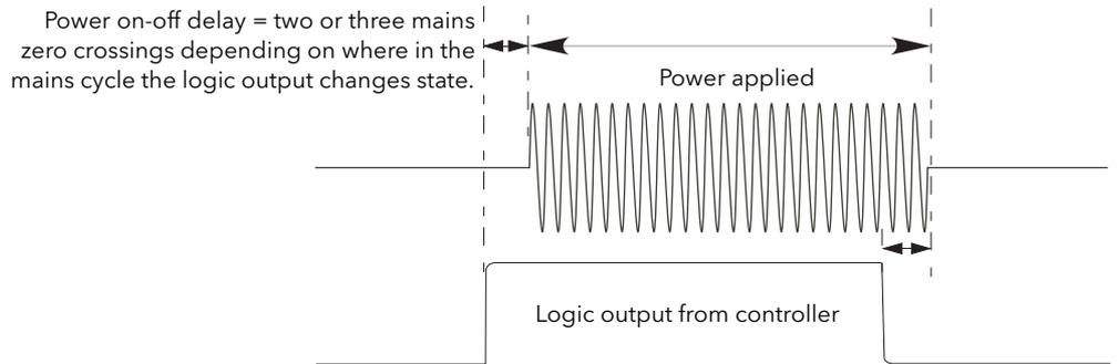
Figure 19 Logic firing mode
