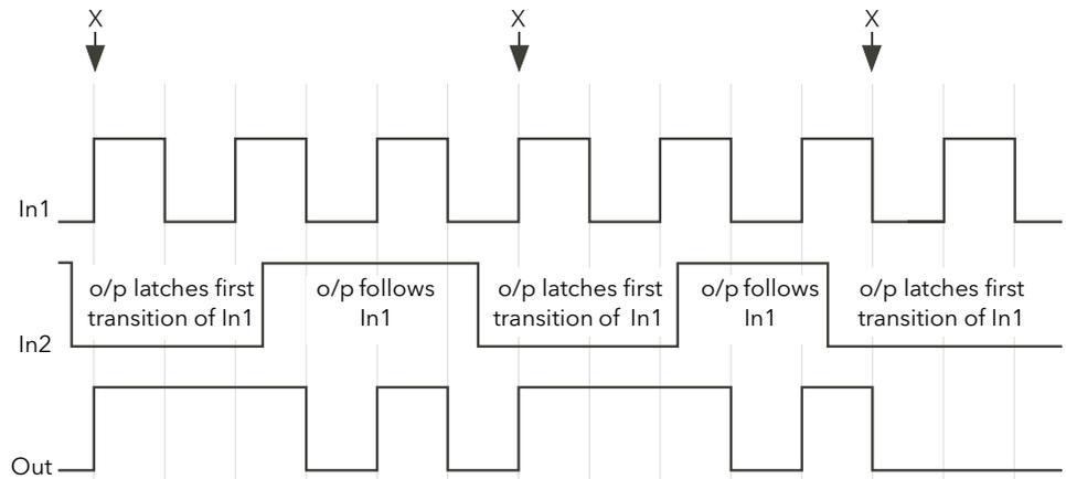
When In2 goes low, Out follows the next positive or negative transition of In1 (points 'X') and latches at this value until In2 goes high. When In2 is high, Out follows In1.
