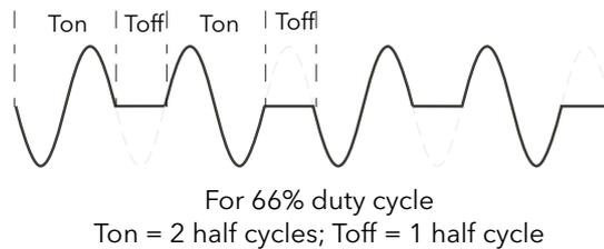
Figure 25 Intelligent half cycle mode: 66% duty cycle
