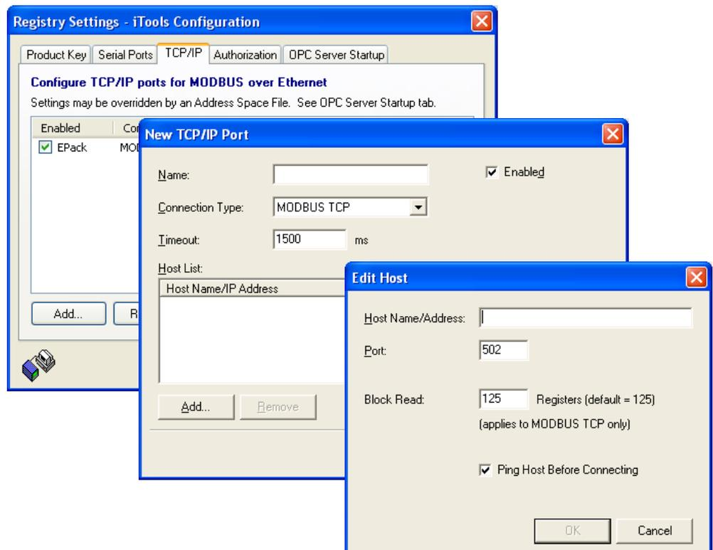
Figure 131 Adding a new Ethernet port
