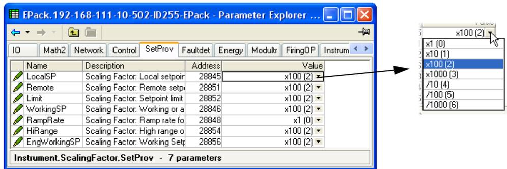
In the above example it can be seen that all the Set point provider parameters are scaled x100, except for Ramp Rate which is not scaled (i.e. the scaling factor = 1). As can also be seen, the scaling factors available are x1, x10, x100, x1000, ÷10, ÷100, ÷1000.
