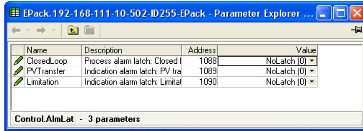
Figure 86 Control Alarm latching page
