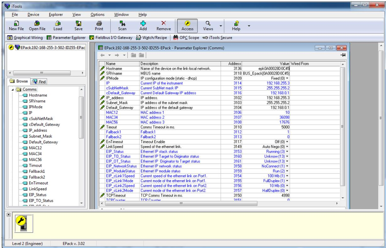
Figure 26 Ethernet/IP User Comms configuration parameters
