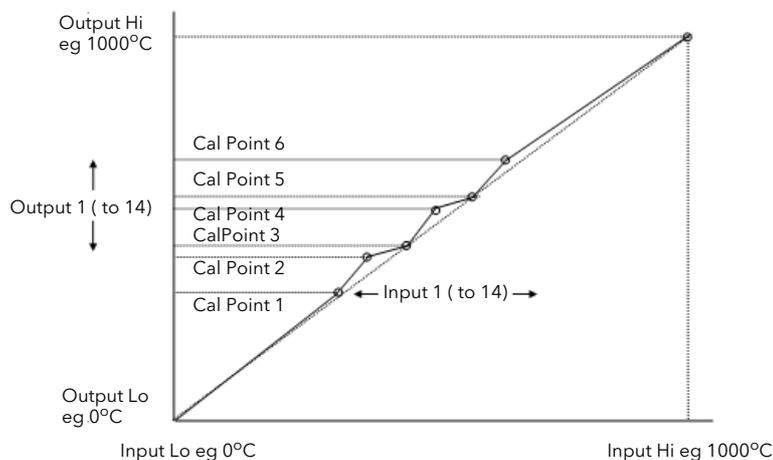
Figure 118 Compensation for Sensor Discontinuities
