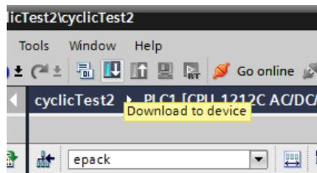
Figure 52 The compiled configuration is downloaded to EPack
