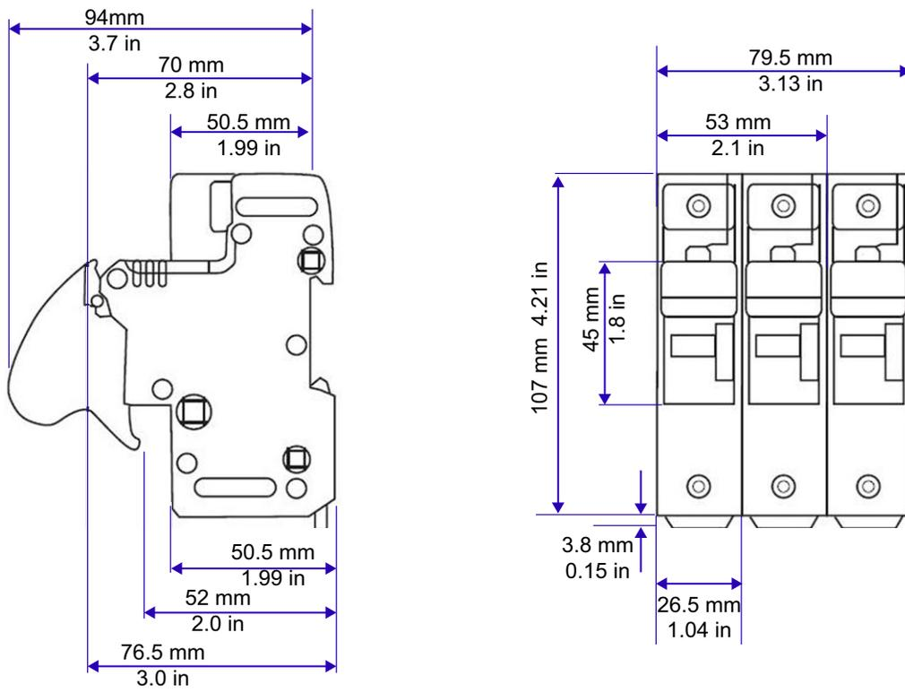
Figure 152 Fuse holder dimensions: US143 (14x51mm)
