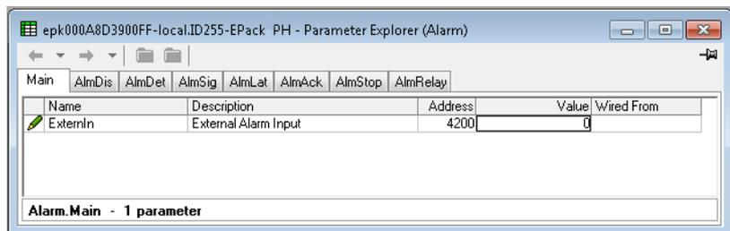
Figure 76 Alarm configuration
