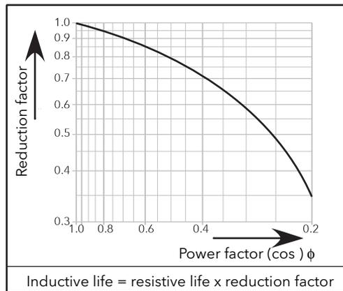
Figure 159 Relay derating curves
