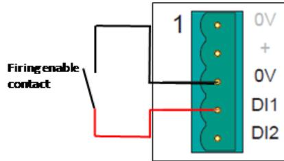
QuickCode menu allows the user to select Digital input 2 to Enable Firing. Digital input 2 is configured in contact closure type, therefore, Firing Enable is achieved by shorting pins 0V and DI2 of the I/O connector located on the underside of the unit (Digital input 2).
