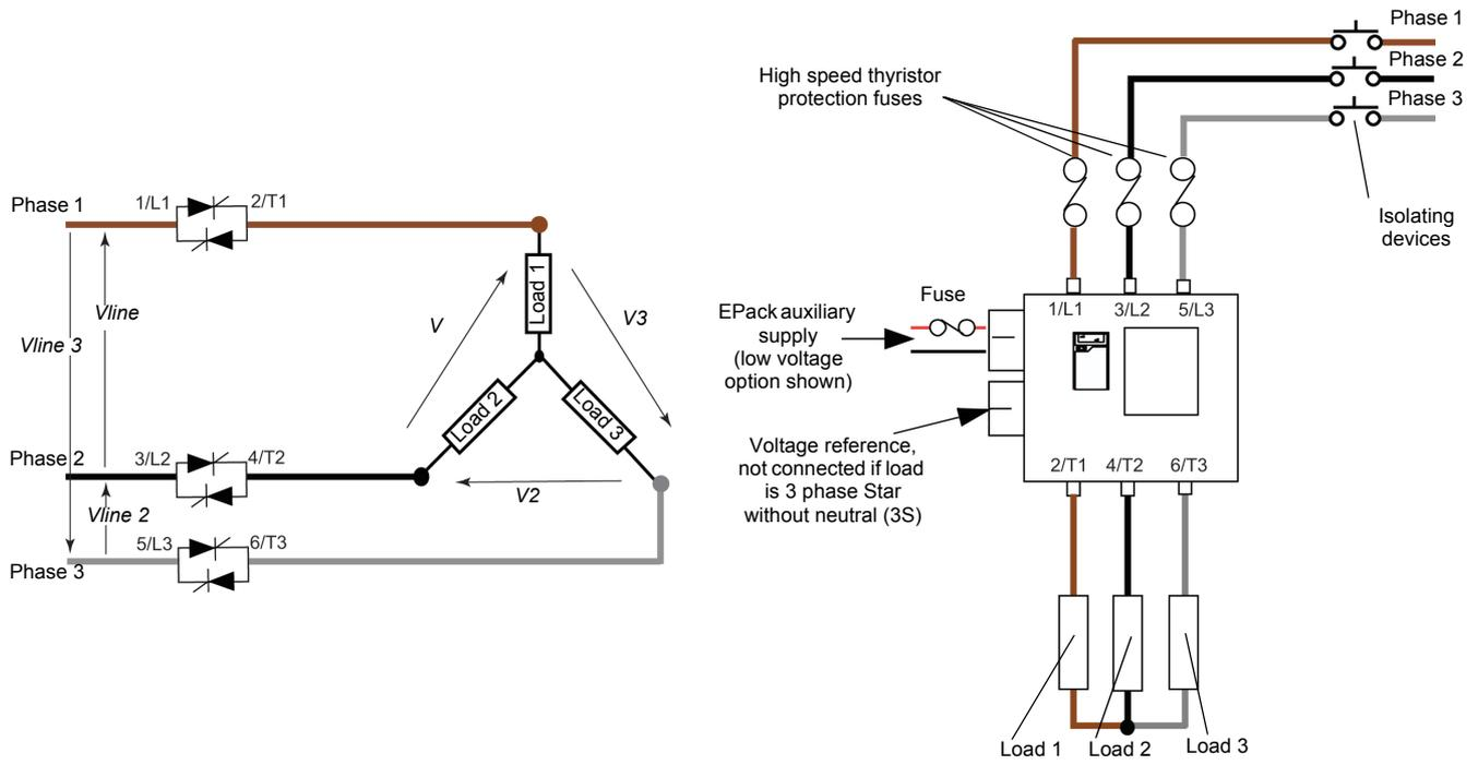
Figure 13 3 phase Star without neutral wiring scheme/load configuration
