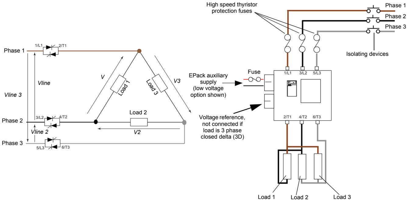
Figure 10 3 phase Closed Delta wiring scheme/load configuration
