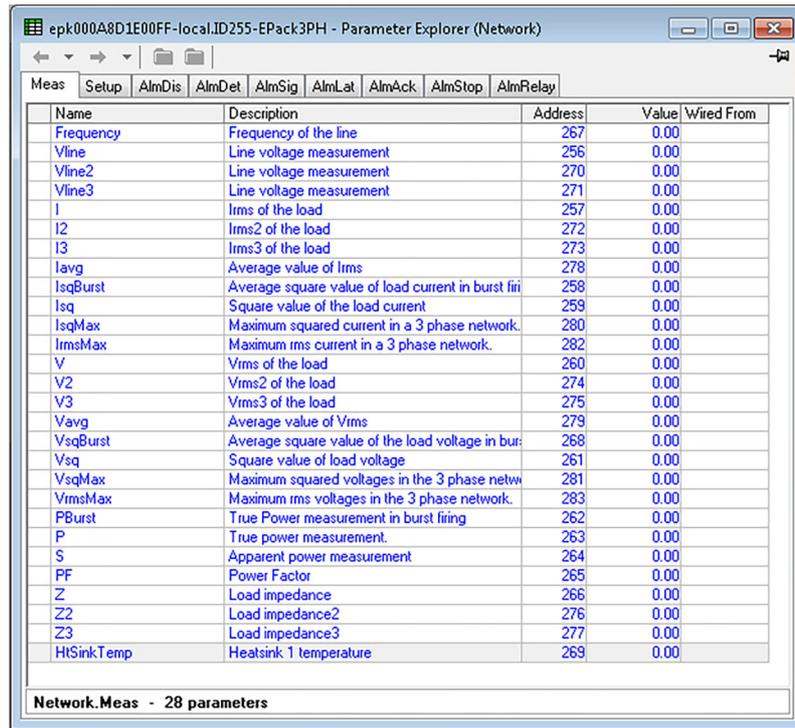
Figure 121 Network, Meas configuration panel
