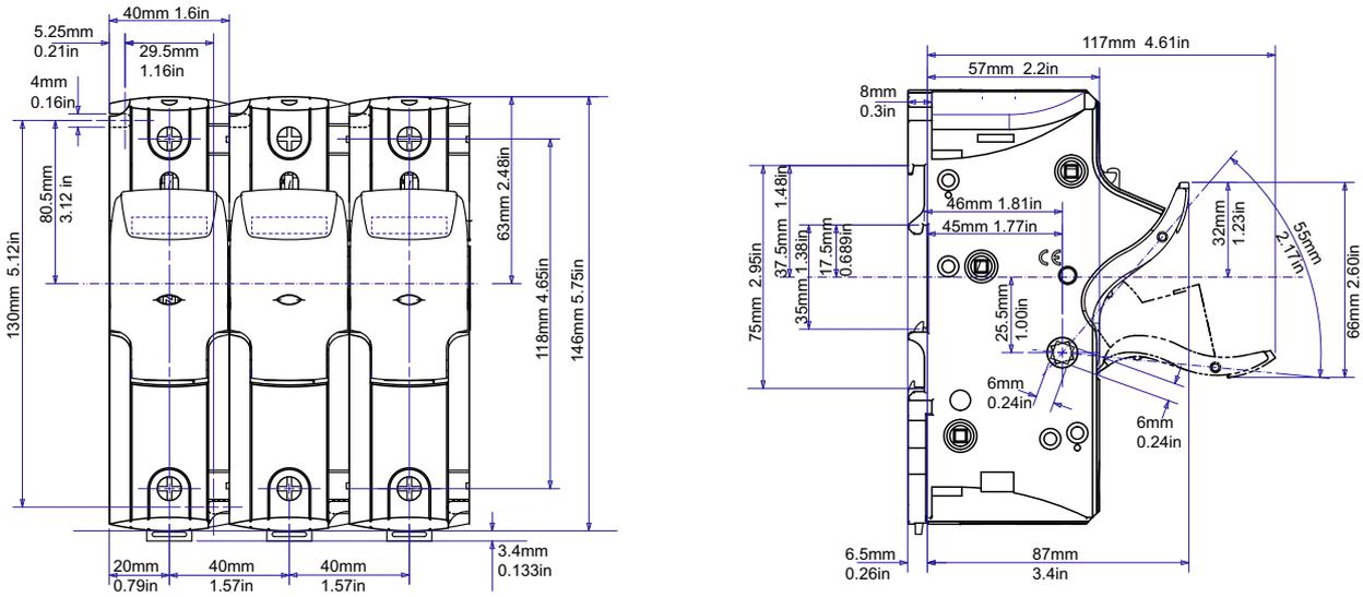
Figure 154 Fuse holder dimensions: US273 (27x60mm)
