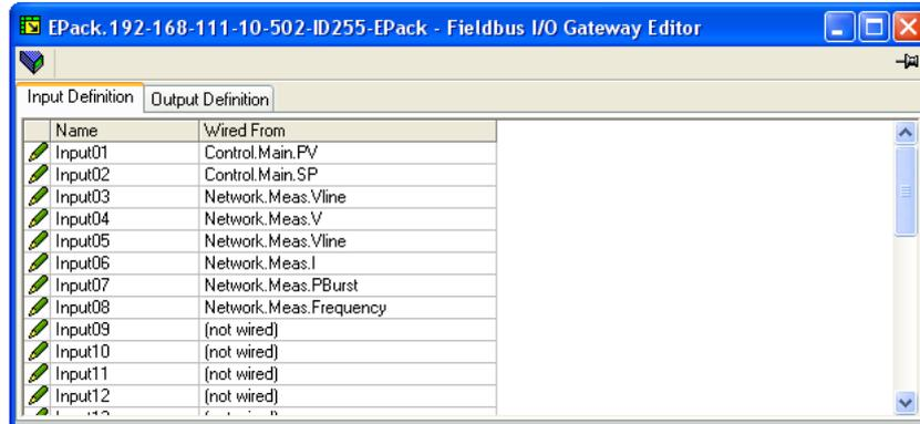
Figure 146 Typical Fieldbus Gateway Parameter list
