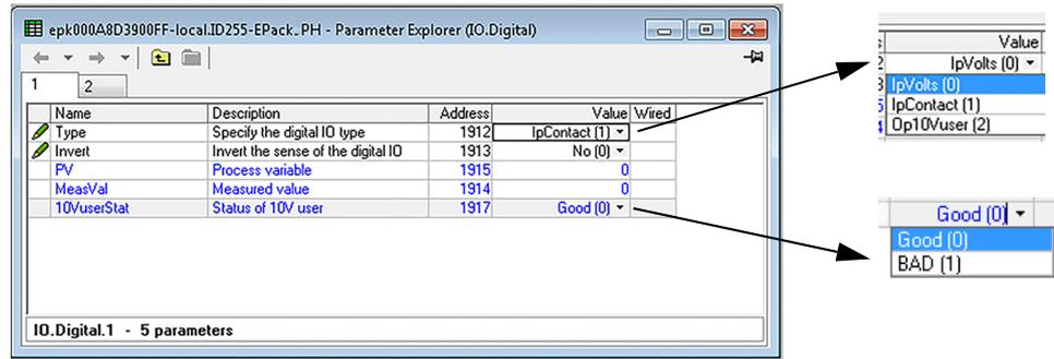
Figure 103 iTools Digital Input configuration page, (digital input 2 displayed)
