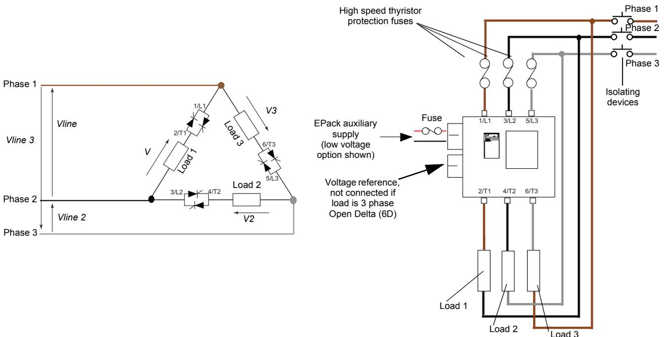
Figure 11 3 phase Open Delta wiring scheme/load configuration
