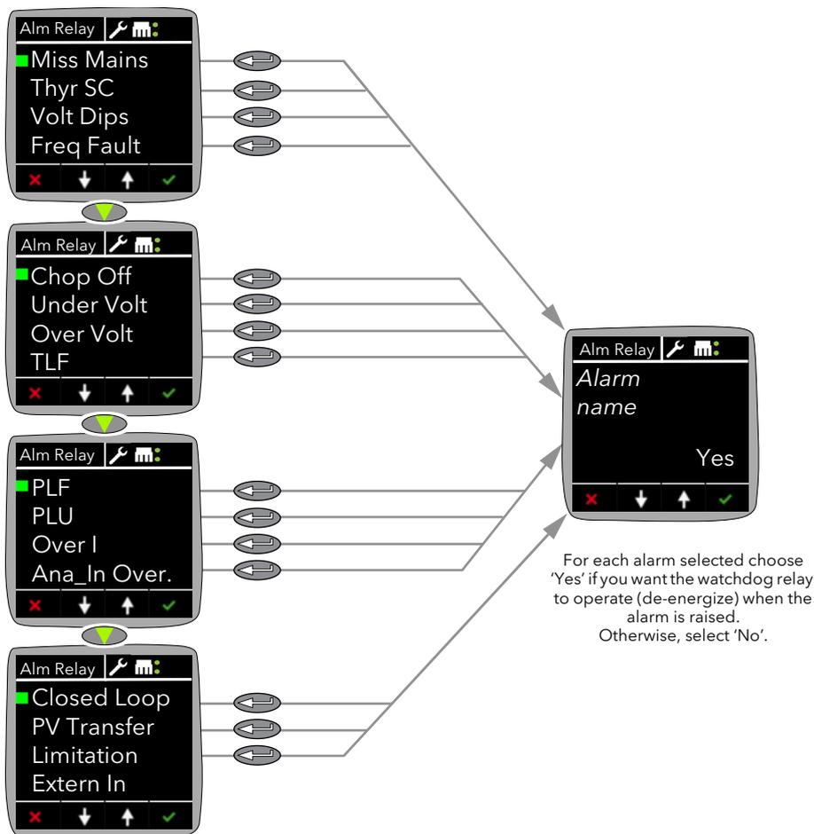
Figure 69 Alarm Relay menu
