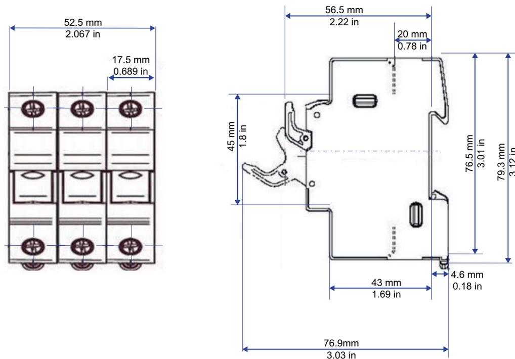
Figure 151 Fuse holder dimensions: CUS103 (10x38mm)
