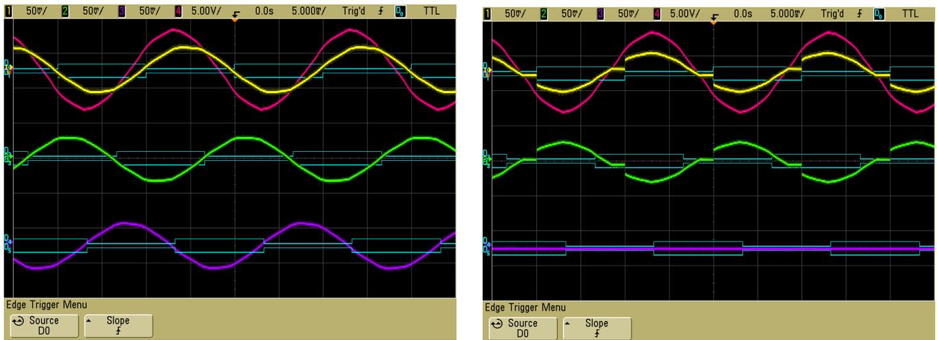
Figure 98 Waveforms; balanced load left, unbalanced load right (ULM off)
