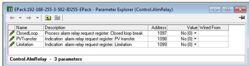
Figure 89 iTools Control Alarm Relay page
