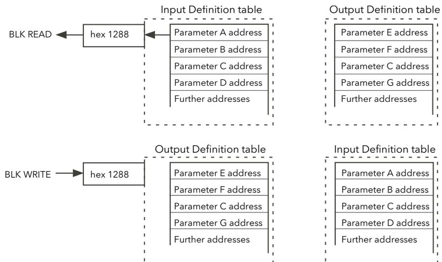
Figure 148 Block read and block write (note 3)
