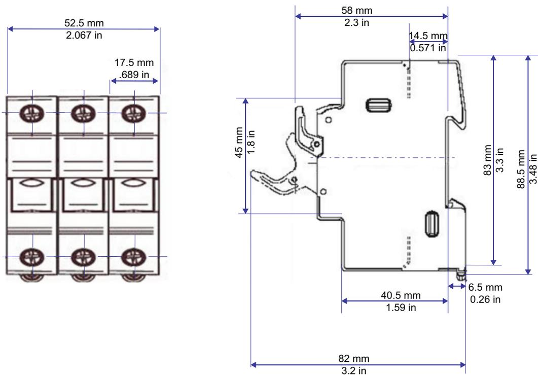
Figure 150 Fuse holder dimensions: US103 (10x38mm)
