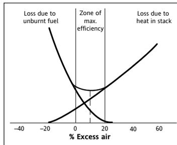
Figure 1 Boiler efficiency
