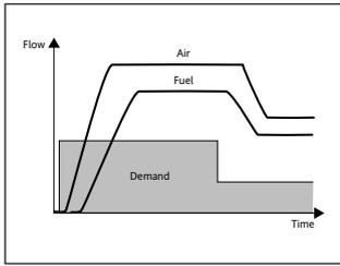
A cross-limiting combustion control strategy ensures that there can never be a dangerous ratio of air and fuel within a combustion process. This is implemented by always raising the air flow before allowing the fuel flow to increase, as shown in Figure 2, or by lowering the fuel flow before allowing the air flow to drop.
