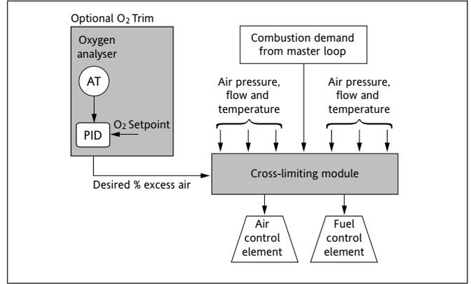
Figure 3 Cross-limiting combustion control with O2 trim
