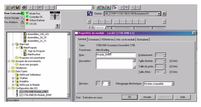
The DeviceNet module is identified with the following symbol: **Module\_DNET**. This identifier will be used later with tools like the Class Instance Editor.
