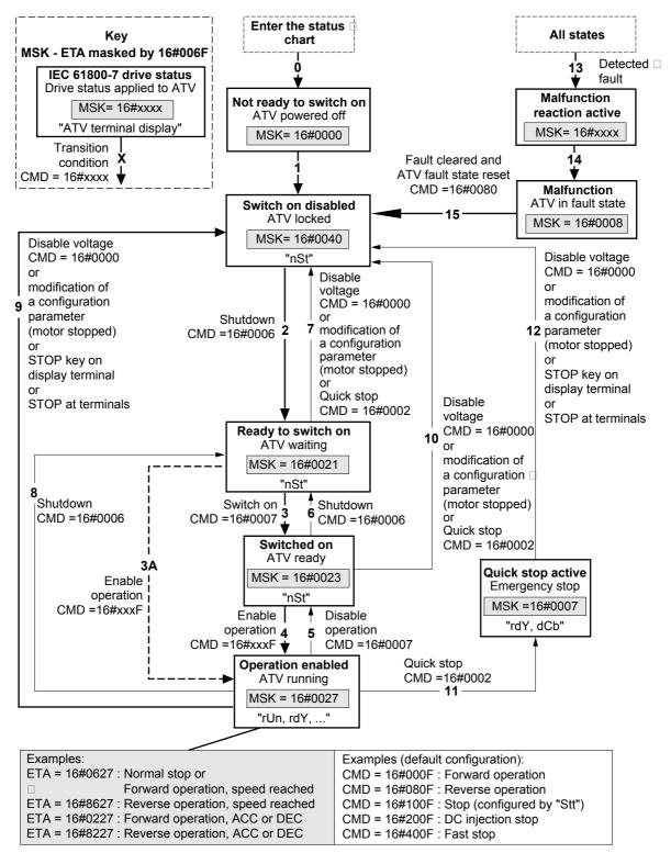
Exiting the "Operation enabled" status via a "Disable voltage" (9) or "Shutdown" (8) command causes a freewheel stop.
