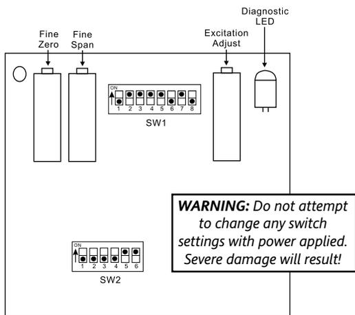
Figure 1: Factory Calibration; 0 to 50mV (calibrated to 0-30mV), 10V excitation, Direct, 4-20mA.
