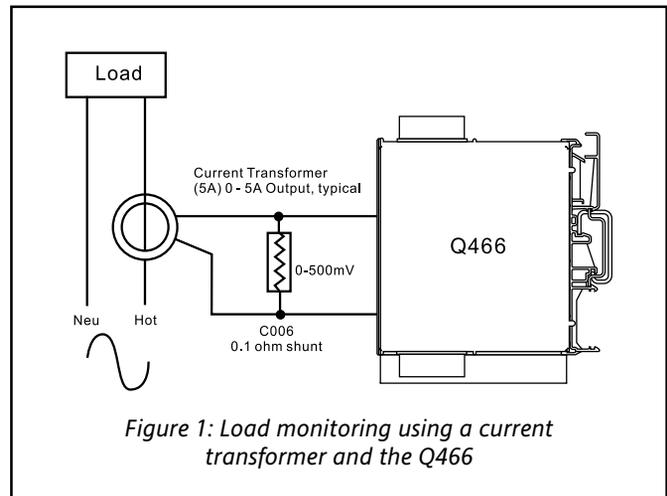
Figure 1: Load monitoring using a current transformer and the Q466
