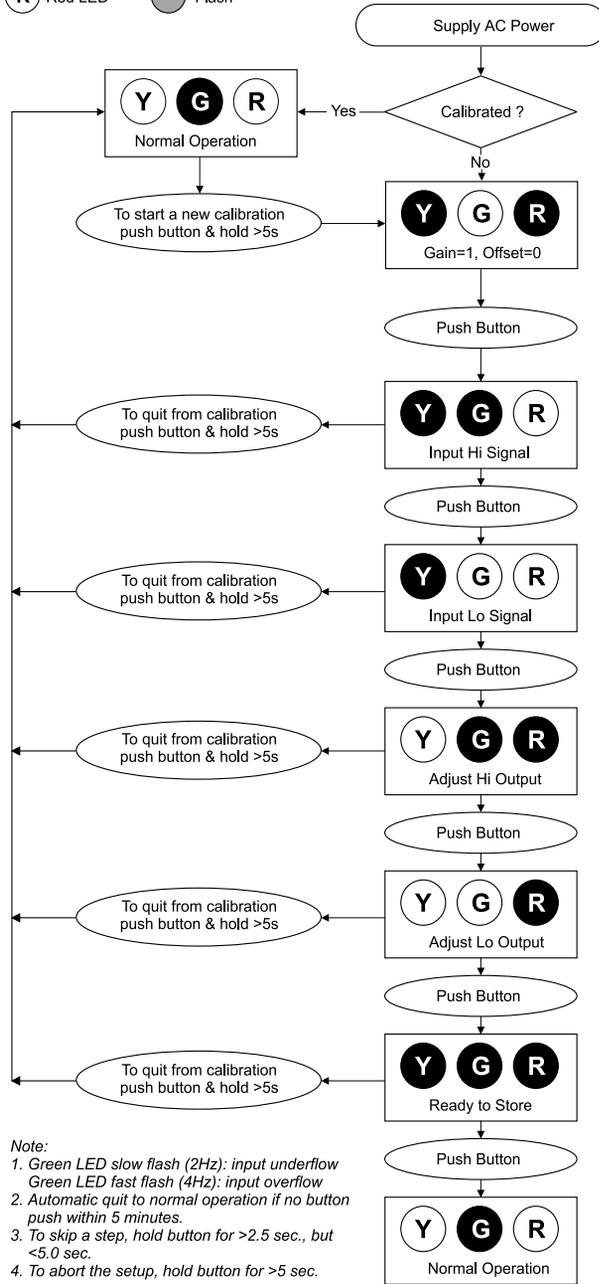
Figure 2: Q406 Calibration Flow Chart
