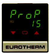
4-digit instrument configuration code (for verification purposes only in this list). The next parameter—the proportional band—can be adjusted as all the others with ▲ and ▼.
