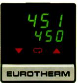
can be freely adjusted within the limits imposed by the SP.Hi and SP.Lo parameters.
