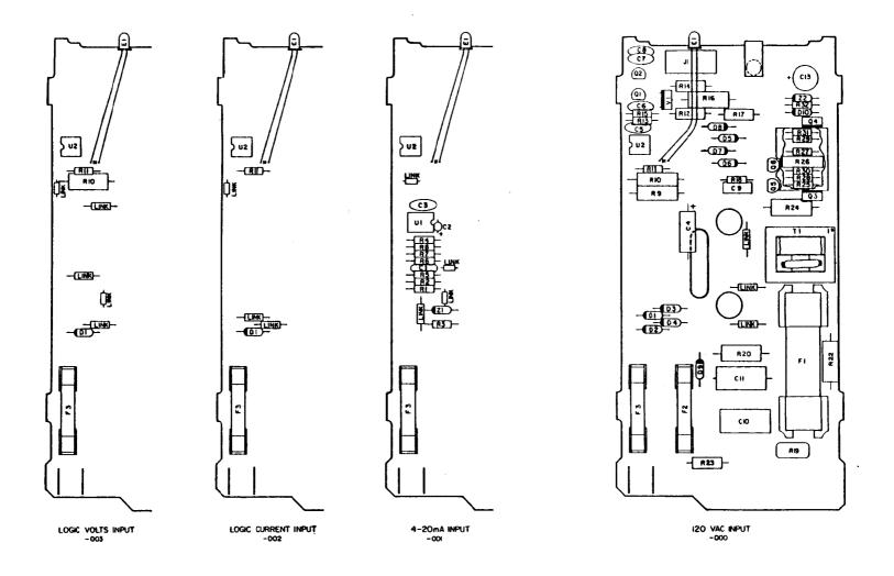
Figure 2.11 831 Triac Control Board Layout (Time Proportioned Inputs)
