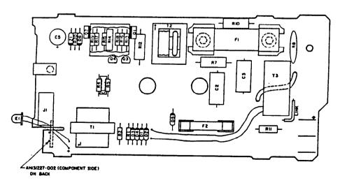
Figure 2.6 831 Triac Control Board Layout
