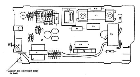
Figure 2.9 831 SCR Control Board Layout
