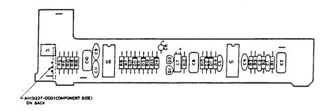
Figure 2.19 831 Phase Angle Sub Board Layout
