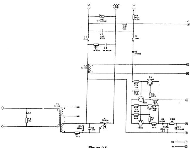
Figure 2.5 831 Triac Control Board Schematic (ZCP Version)
