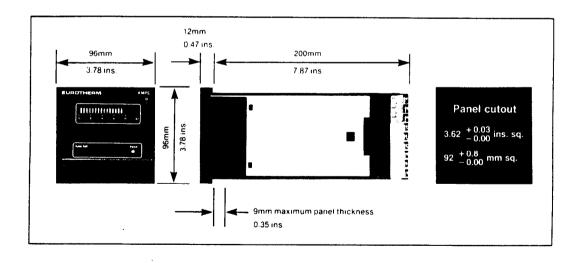
Figure 3.1 Model 831 SCR Dimensions
