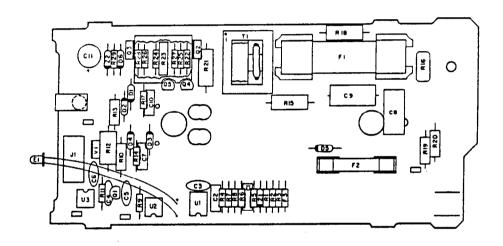
Figure 2.17 831 SCR Control Board Layout (4-20mA-PA Input Version)
