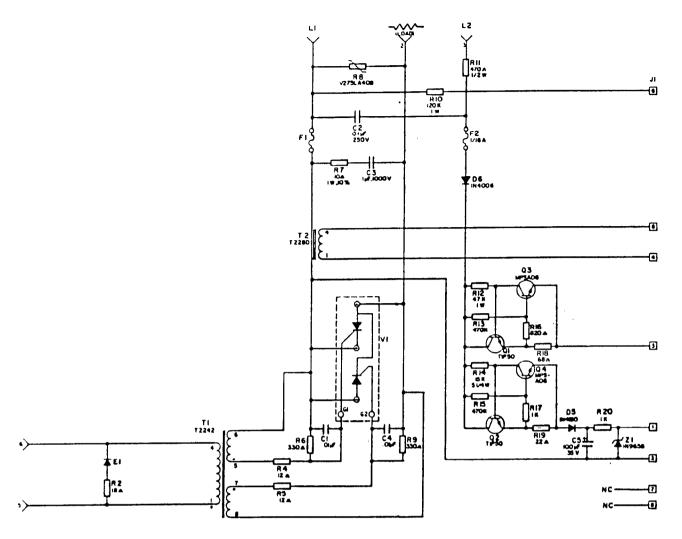
Figure 2.8 831 SCR Control Board Schematic (ZCP Version)
