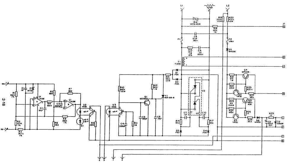
Figure 2.16 831 SCR Control Board Schematic (4-20mA-PA Input Version)
