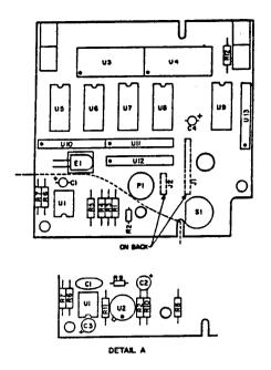
Figure 2.3 831 Display Board Layout
