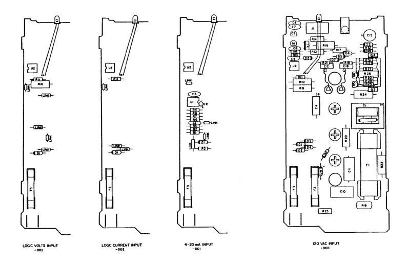
Figure 2.13 831 SCR Control Layout Board (Time Proportioned Inputs)
