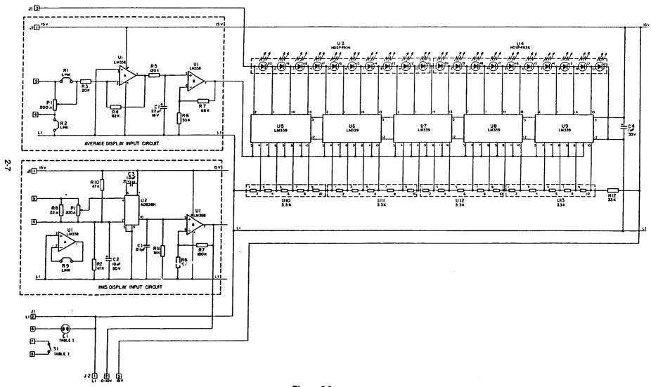
Figure 2.2 831 Display Board Schematic
