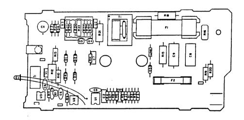
Figure 2.15 831 Triac Control Board Layout (4-20mA-PA Input Version)
