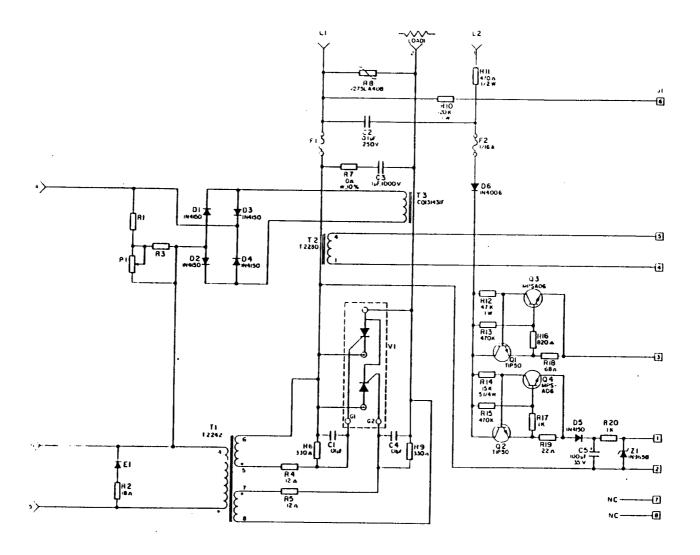
Figure 2.7 831 SCR Control Board Schematic (PAP Version)
