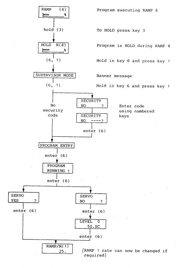
Scroll through the parameters pressing key 6 and action any changes using the  $\nabla\Delta$  keys. Press key 1 to return to the HOLD segment at any time.
