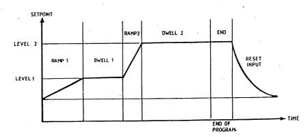
During a program run parameters can be inspected but not altered. When an active dwell period is being inspected the time to the end of the dwell period is monitored. If a dwell parameter is inspected when the programmer is not in that segment the original full dwell period is displayed.
