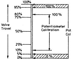
To calibrate the potentiometer to the motor travel connect up the instrument as described in the wiring instructions. Scroll through until 'Pc' is displayed. Simulataneously depress the UP, DOWN and SCROLL buttons and an 'H' and a value will be displayed. This signifies the high limit value of the motor travel.
