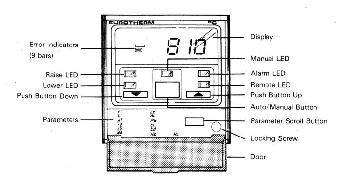
INSTRUMENT DESPATCHED WITH PARAMETER SCROLL BUTTON DISABLED
