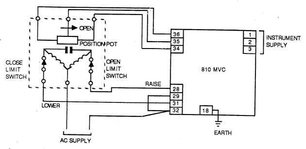
Connection to motor without position potentiometer fitted.
