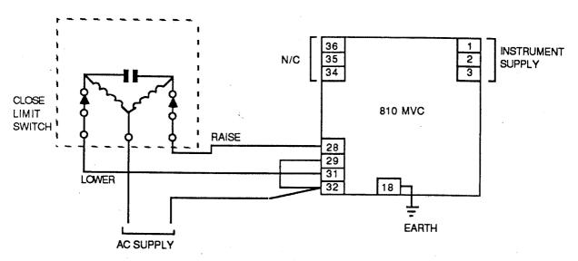
Connection to motor with external raise and lower buttons acting directly on motor.
