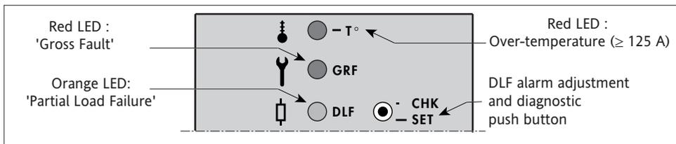
Figure 3-1 Layout of front panel LEDs with 'DLF' option
