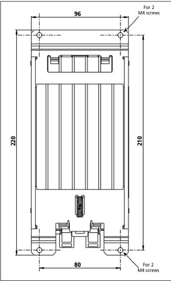
Figure 2-2 Bulkhead mounting - 16 A to 63 A units
