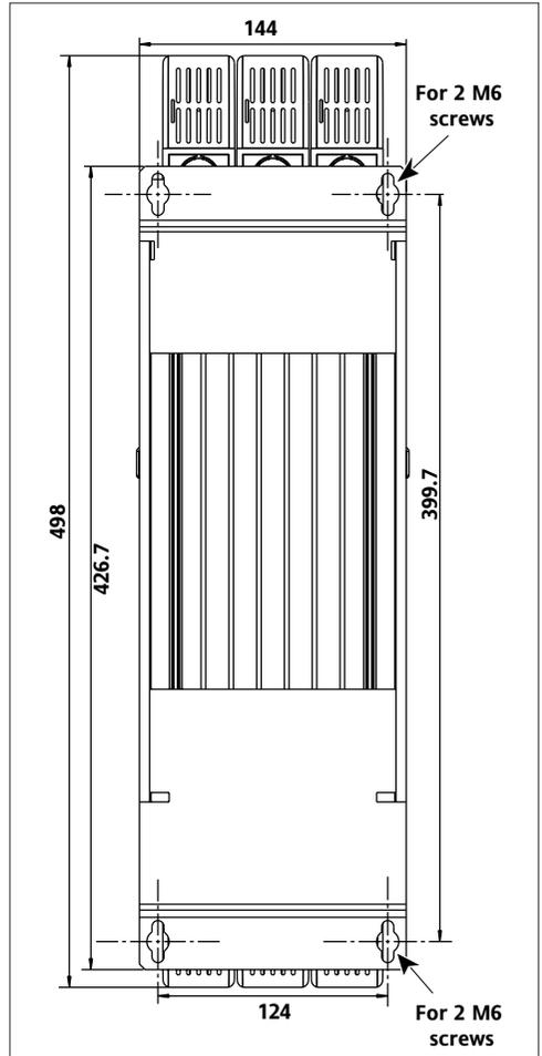
Figure 2-4 Bulkhead mounting -  $\geq$  125 A units
