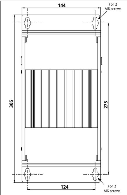
Figure 2-3 Bulkhead mounting - 80 A to 100 A units
