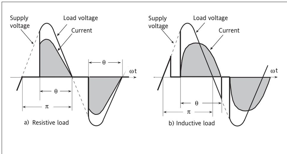
Figure 3-5 Voltage and current in 'Phase angle' mode
