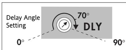
To avoid the over-current, the **first thyristor firing** must be **delayed** relative to the corresponding zero for each phase.
