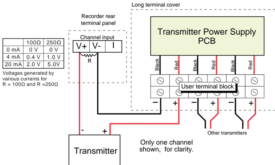
R (minimum spec) = 1.4W, ± 1%. 100Ω or 250Ω as required (see table)
