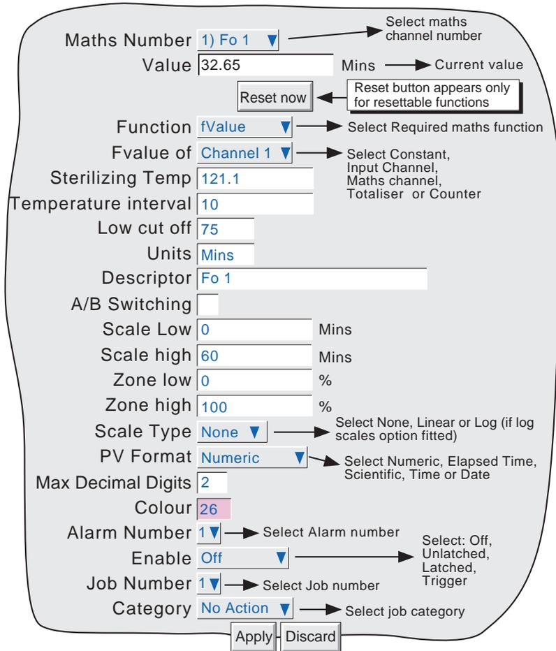
Figure 3.1 Maths configuration menu (typical - varies from function to function)
