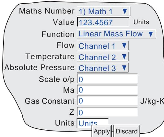
Figure 3.2.3 Linear mass flow menu
