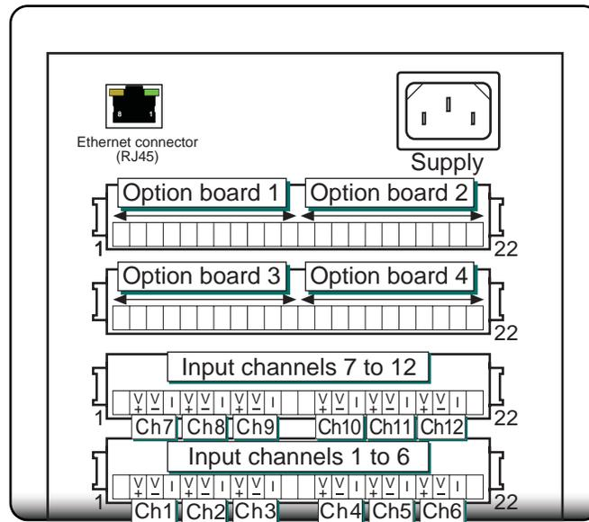
Figure 10.1.2a Back panel connector details.
