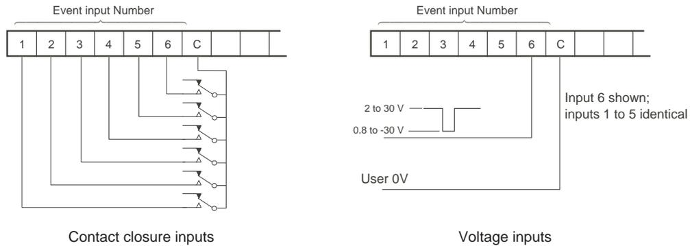
Figure 7.3 Event input wiring (discrete inputs)
