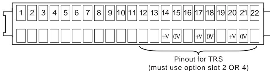
Figure 10.2 TRS pinout
