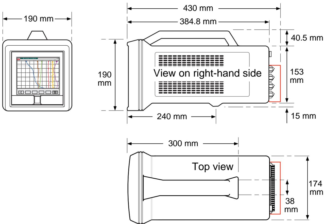
Figure 10 Portable case dimensions
