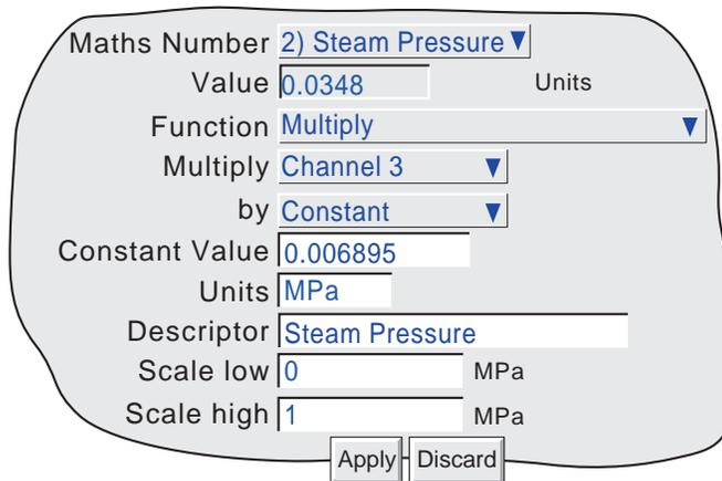
Figure 3.2.7b PSI to MPa conversion example
