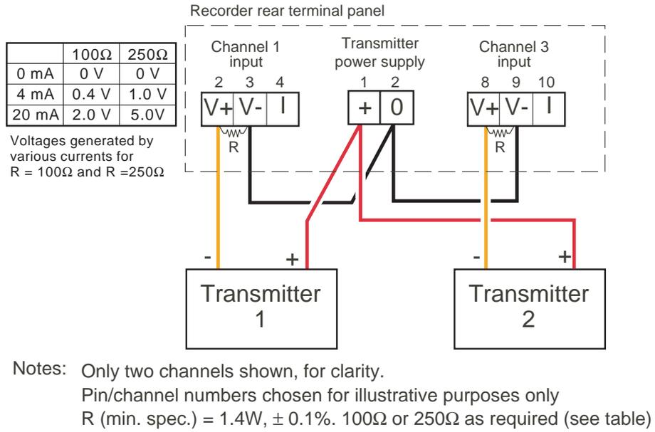
Figure 9.3 Typical transmitter wiring
