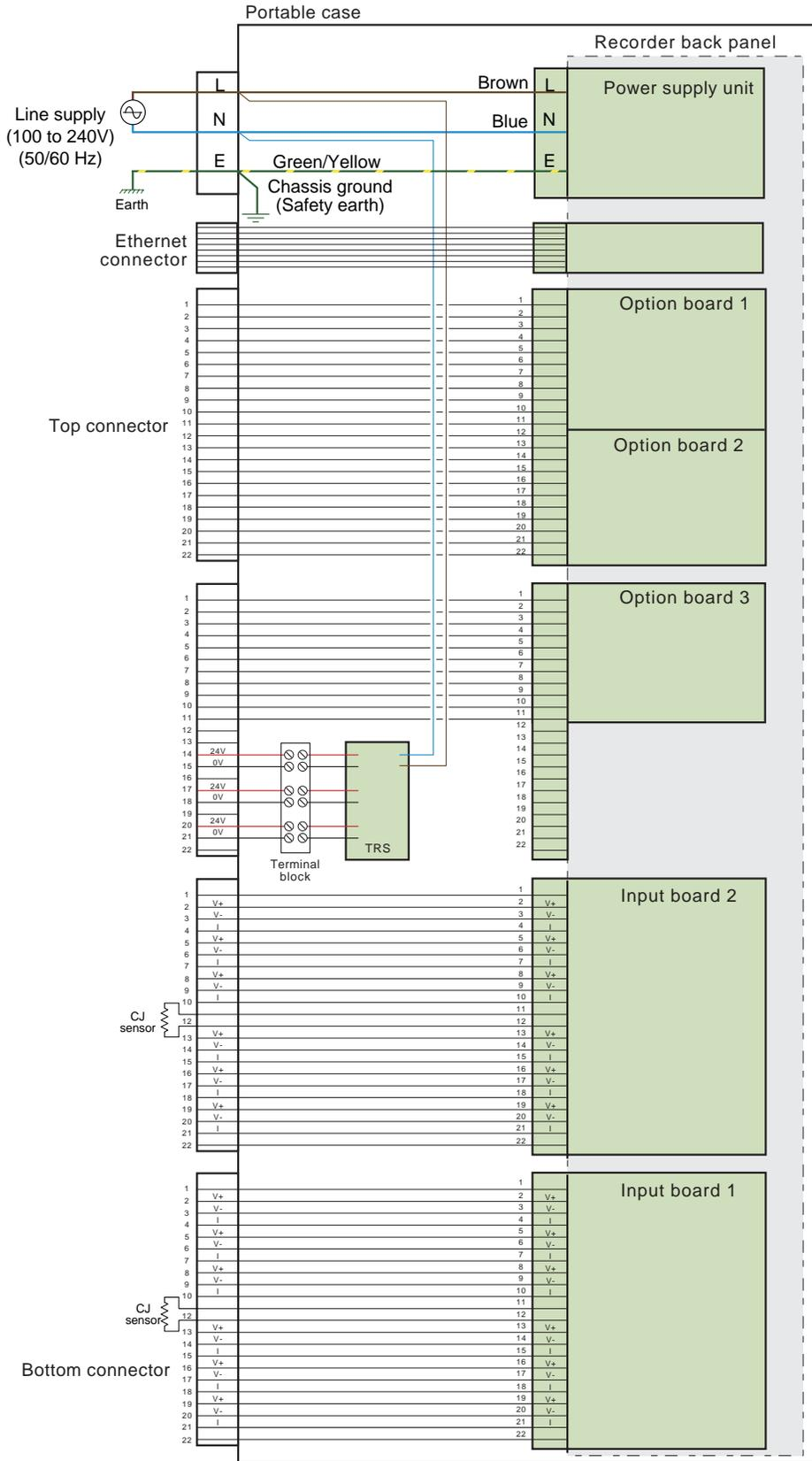
Figure 10.2.1 Typical internal wiring
