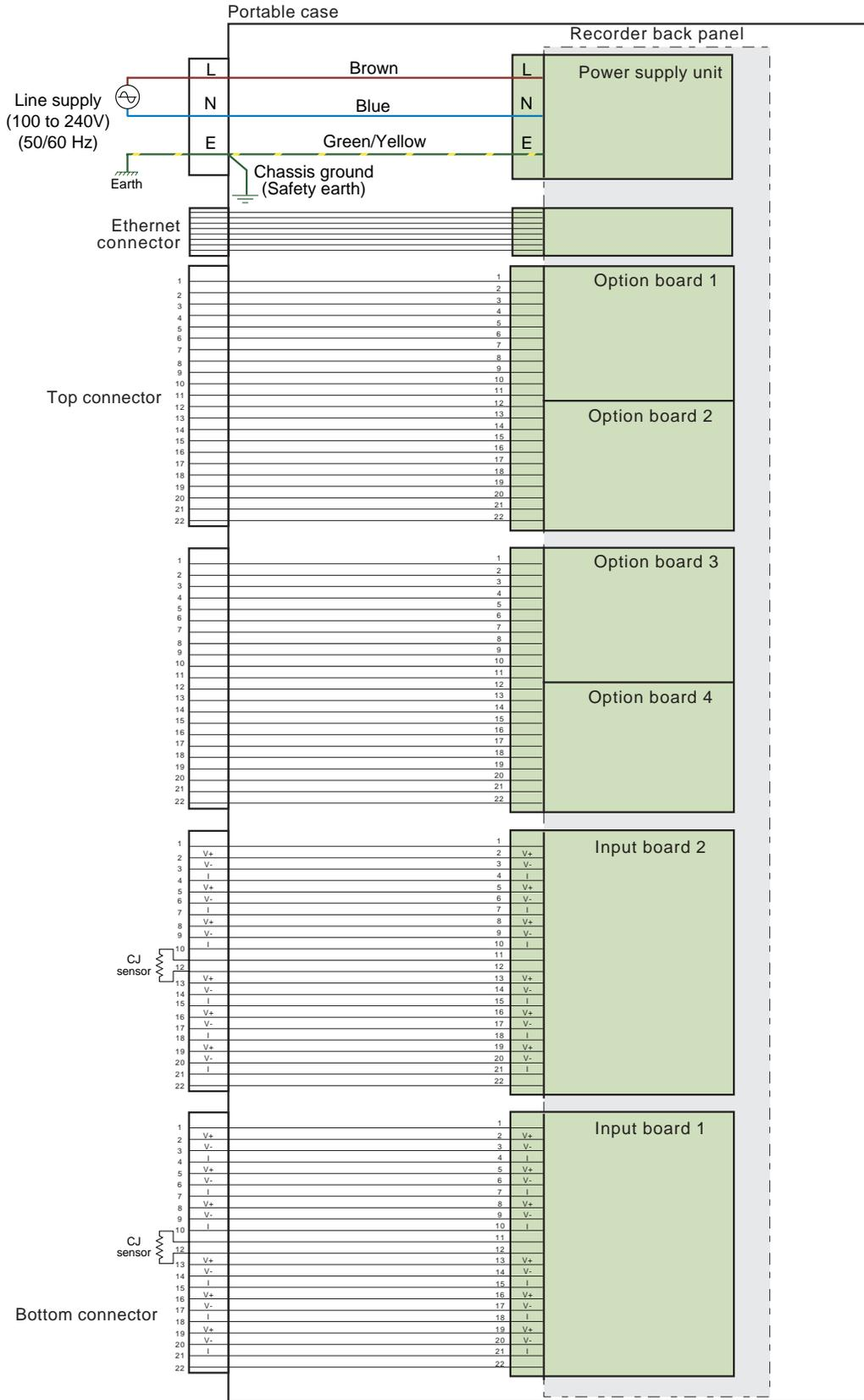
Figure 10.1.2b Basic option internal wiring
