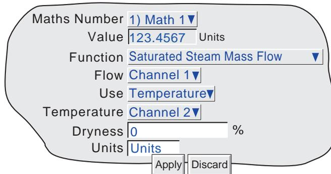
Figure 3.2.7a Typical Saturated Steam Mass Flow configuration page
