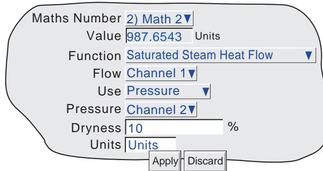
Figure 3.2.8 Typical Saturated Steam Heat Flow configuration page
