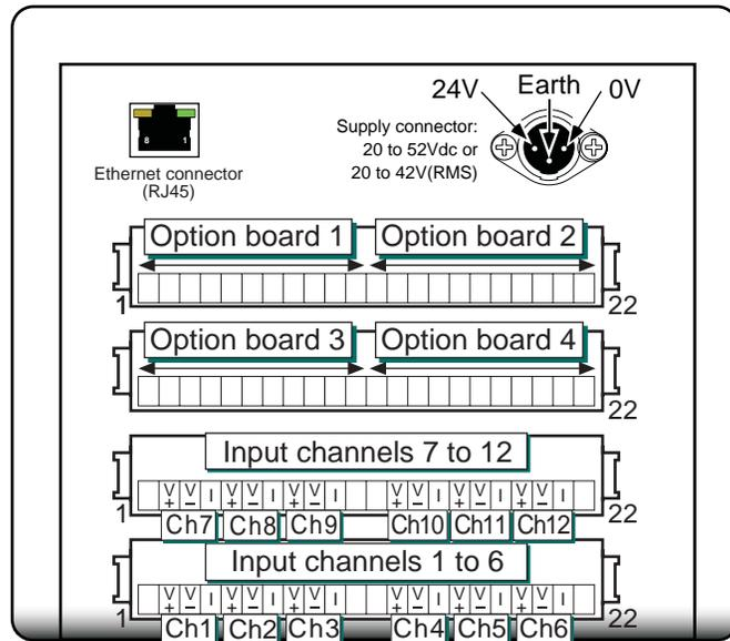
Figure 10.5b Low supply voltage connector details
