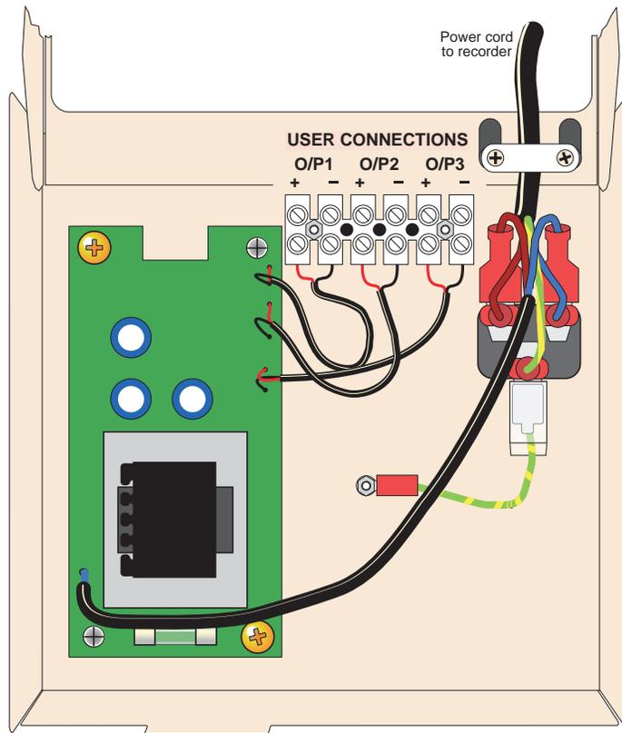
Figure 8.2.3a Terminal block wiring
