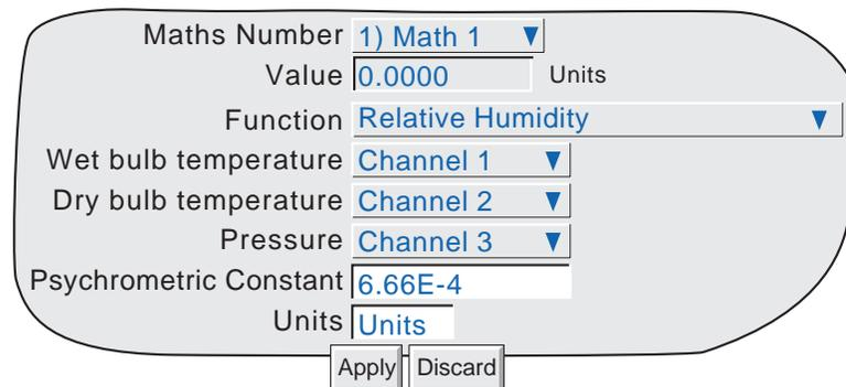
Figure 3.2.13 Relative humidity configuration menu
