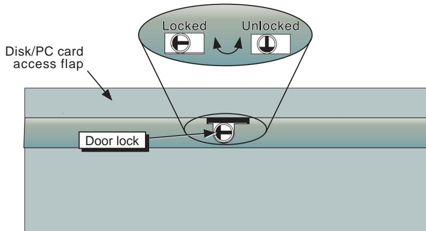
Figure 12b Door lock detail - 180 mm recorder
