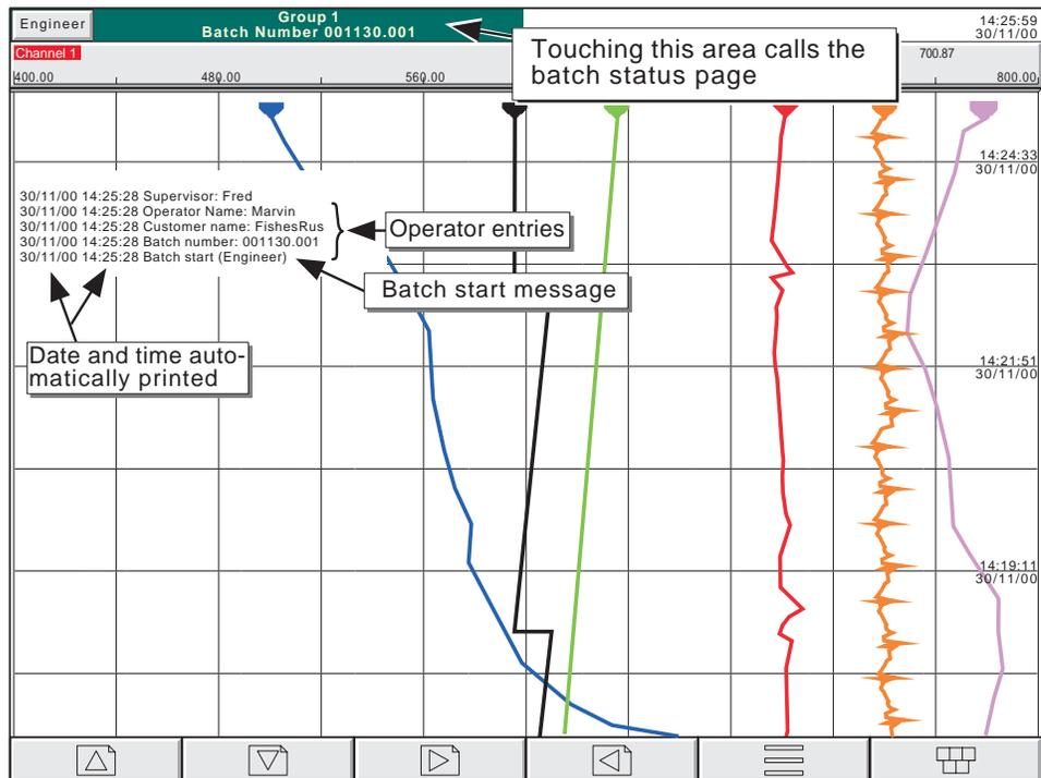
Figure 1.3.1c Typical Batch start messages
