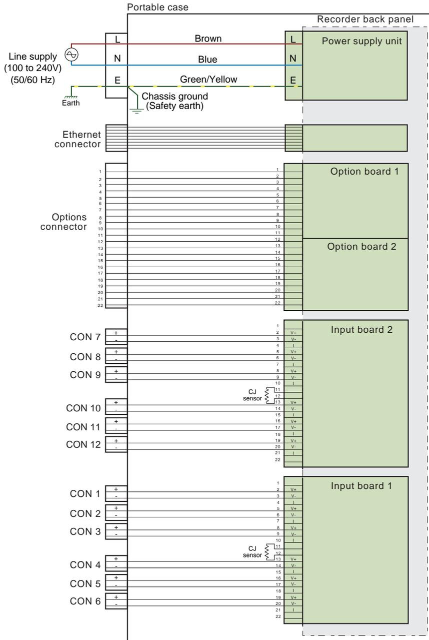
Figure 10.4.2c Internal wiring
