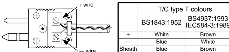
Figure 10.3.2b Thermocouple plug wiring (cover removed for clarity)
