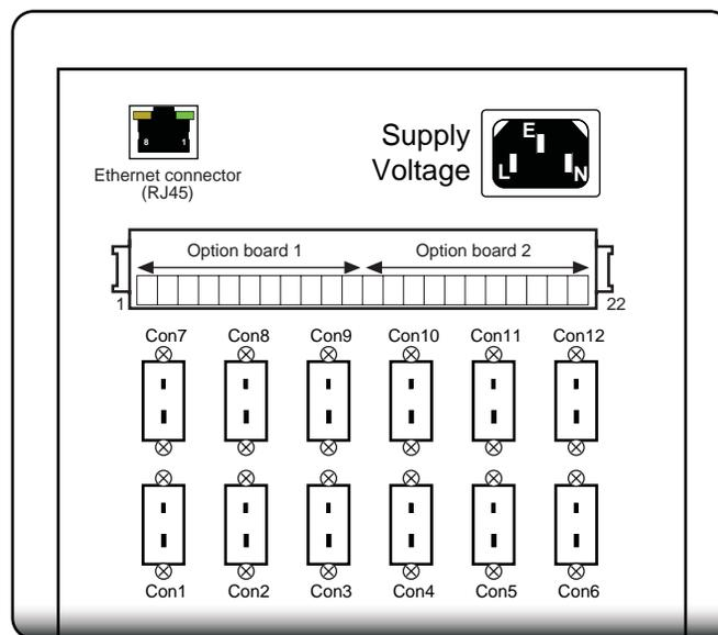
Figure 10.4.2a Rear panel connector locations
