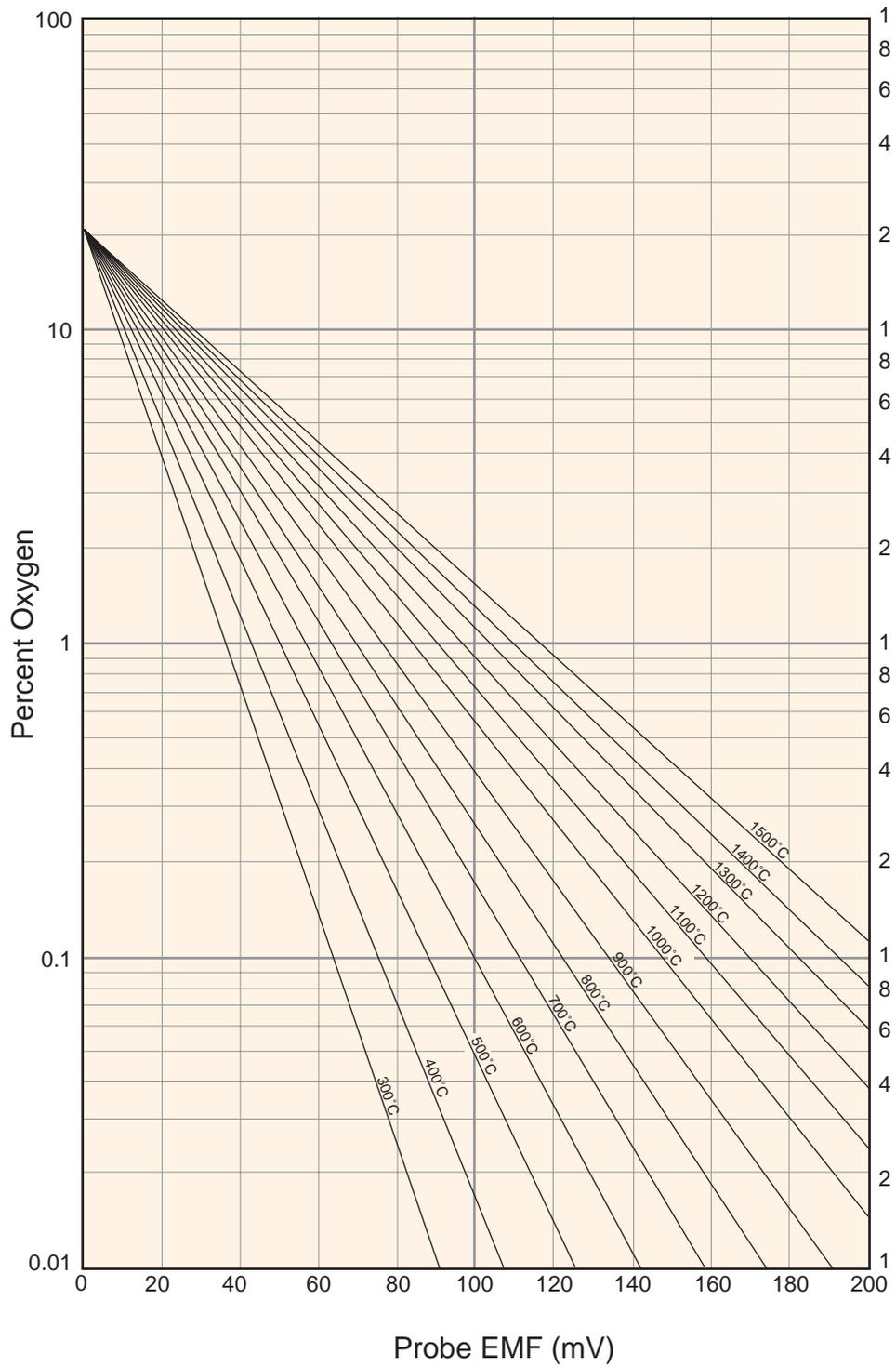
Figure 3.2.14b Probe emf versus temperature
