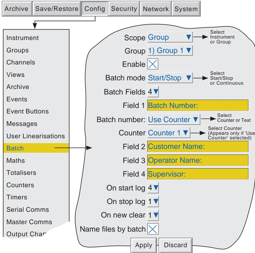
Figure 1.2 Batch configuration menu
