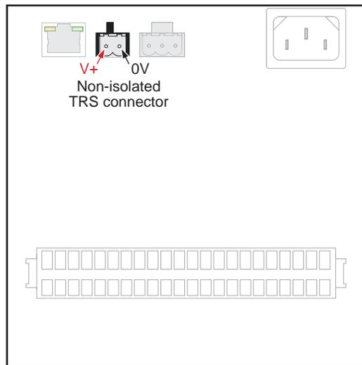
Figure 9.2 Connector location and pinout
