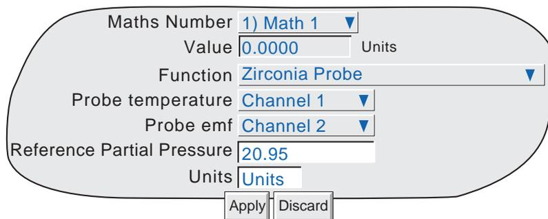
Figure 3.2.14a Zirconia probe function configuration menu
