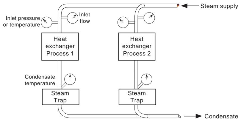
Figure 3.2.9a Measurement transducer - typical locations
