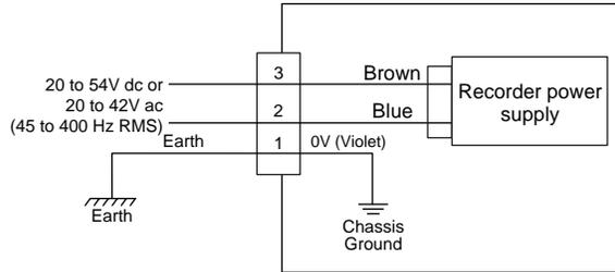
Figure 10.5a Internal wiring for low voltage options
