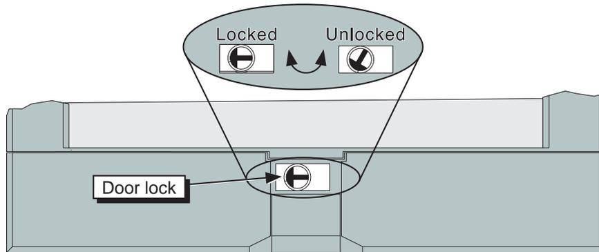
Figure 12a Door lock detail - 100 mm recorder
