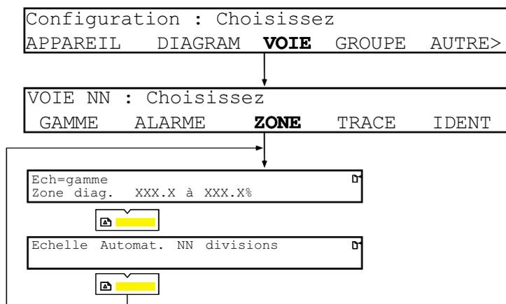
Figure 4.4.4 Channel configuration: Zone
