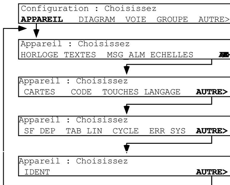
Figure 4.2 Configuration appareil
