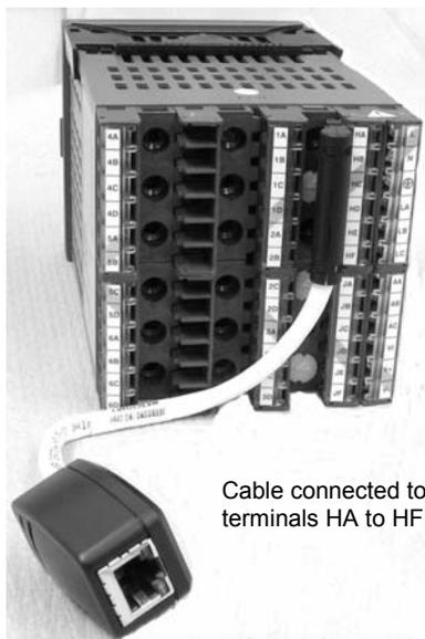
Cable connected to terminals HA to HF
