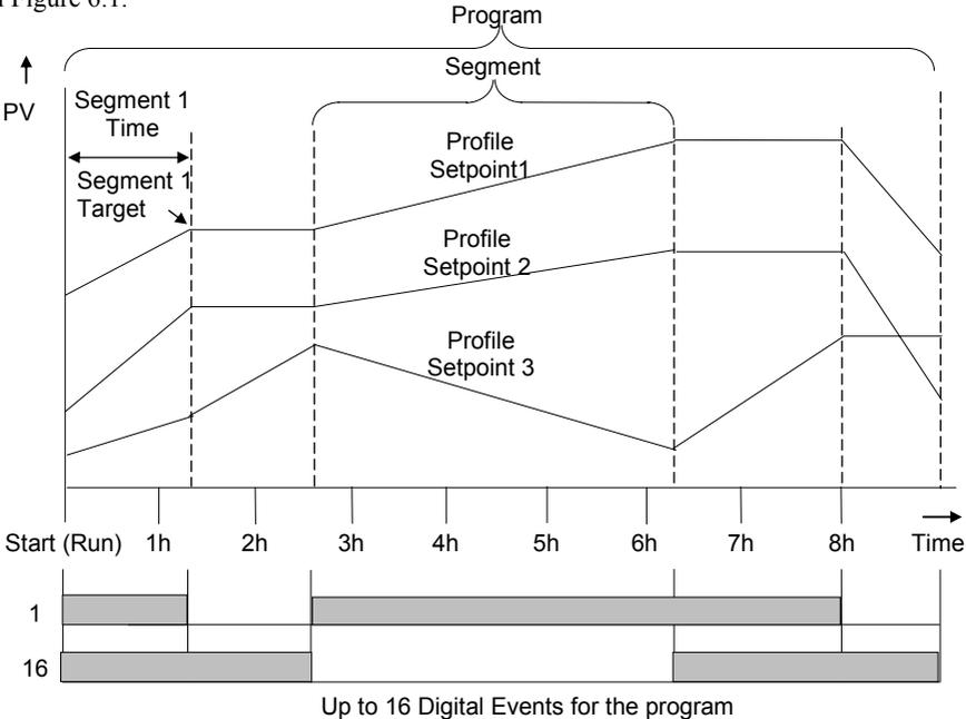
Figure 4-1: An Example of a Synchronous Setpoint Program
