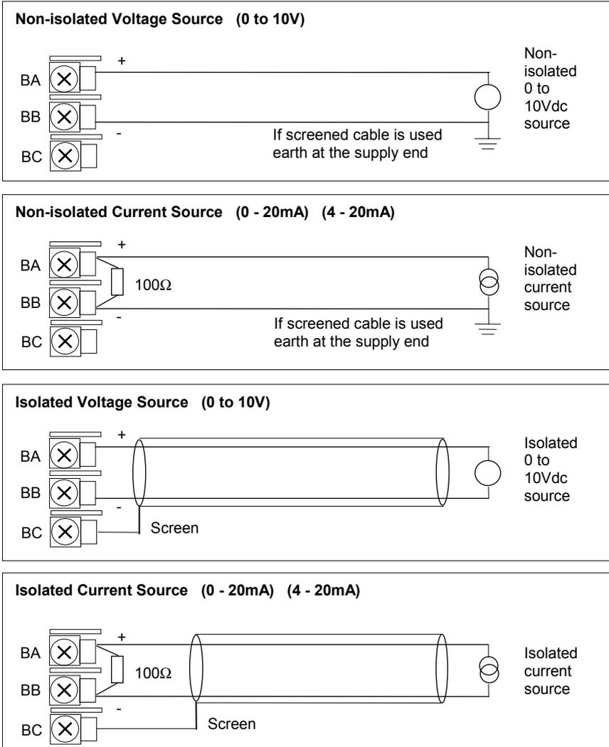
Figure 2-7: Wiring Connections For Analogue Input
