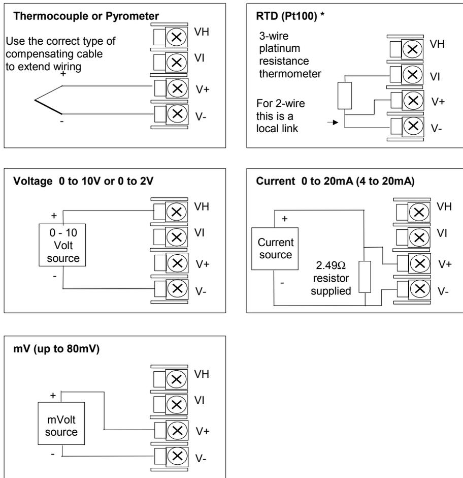
\* Note: This connection is shown for 26 and 2700 series controllers. It is not the same as 2400 and 2200 series controllers.
