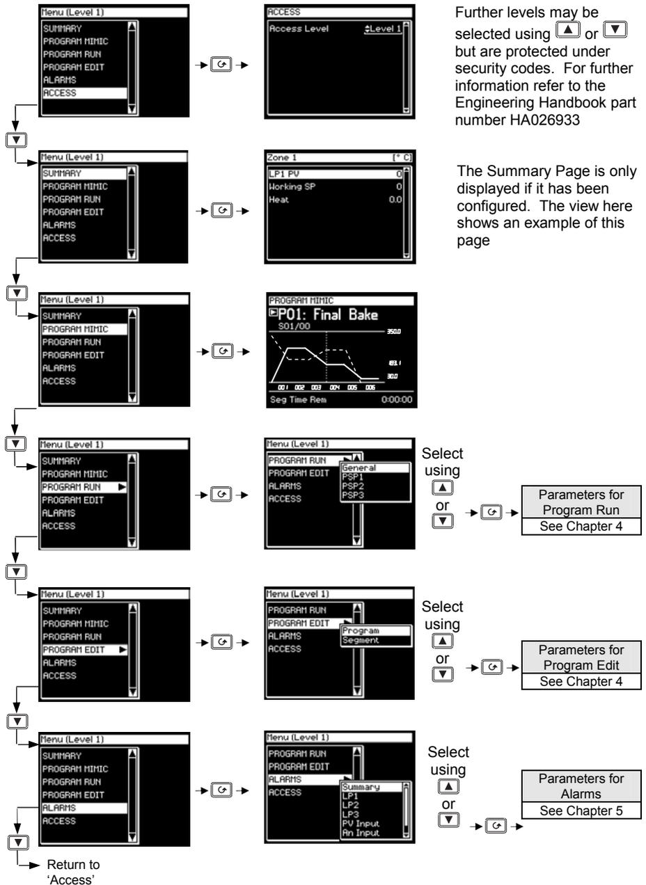
Figure 3-7: Navigation Diagram
