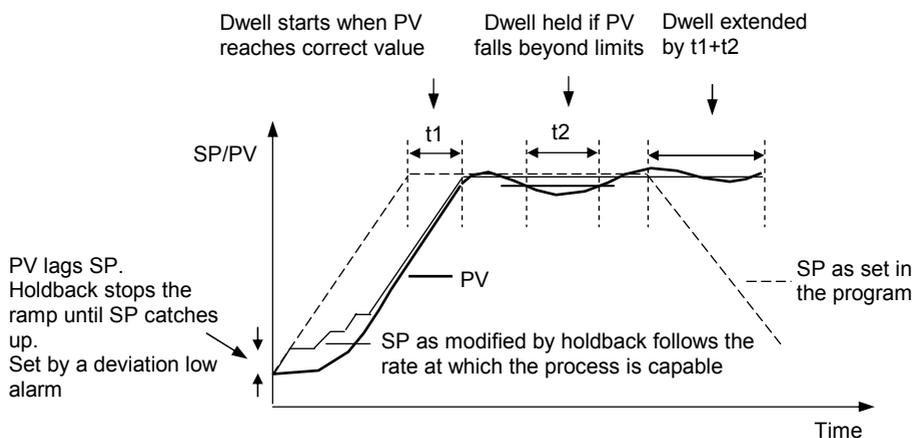
Figure 4-3: Effect of Holdback to Produce Guaranteed soak
