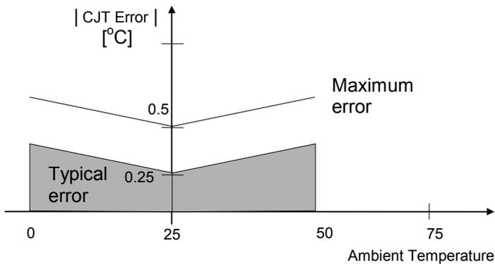
**Figure C-5: Overall CJT Error at Different Ambient Temperatures**
