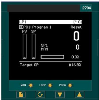
← A flashing bar underlines the selected parameter (output power)
