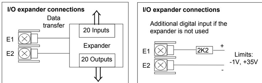
Figure 2-8: Wiring Connections for the I/O Expander
