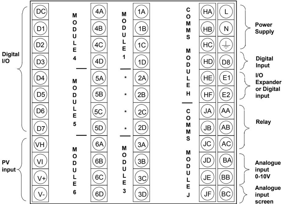
The functionality of the two outer rows of terminals is common to all instrument variants, as follows:-
