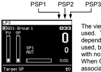
The view shown here is applicable when Groups are used. The number of displayed status symbols depends on the number of programmer blocks used, but the order of display is always left to right – with no gaps. When Groups are not used the program status is associated with the individual loop pages.
