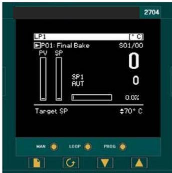
← A flashing bar underlines the selected parameter (setpoint)
