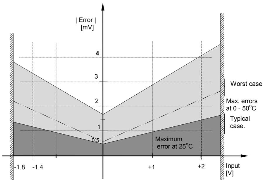
Figure C-2: Error Graph - 0 - 2V Input
