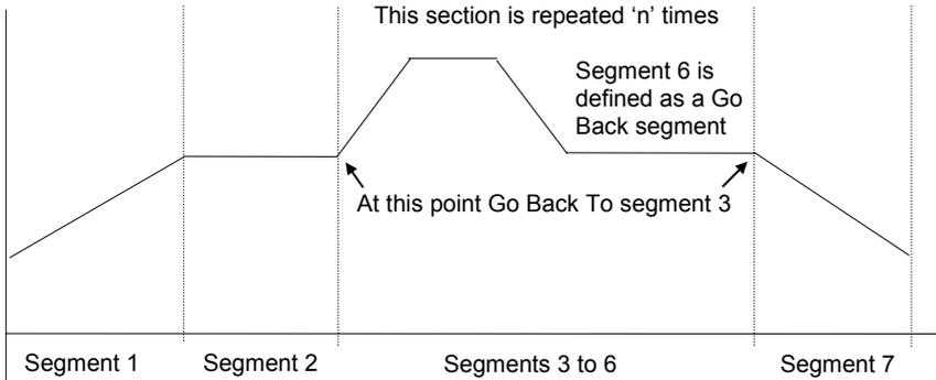
**Figure 4-5: An Example of a Program with Repeating Section**
