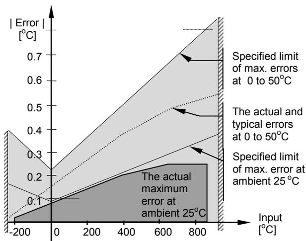
Figure C-4: Error Graph - RTD Input
