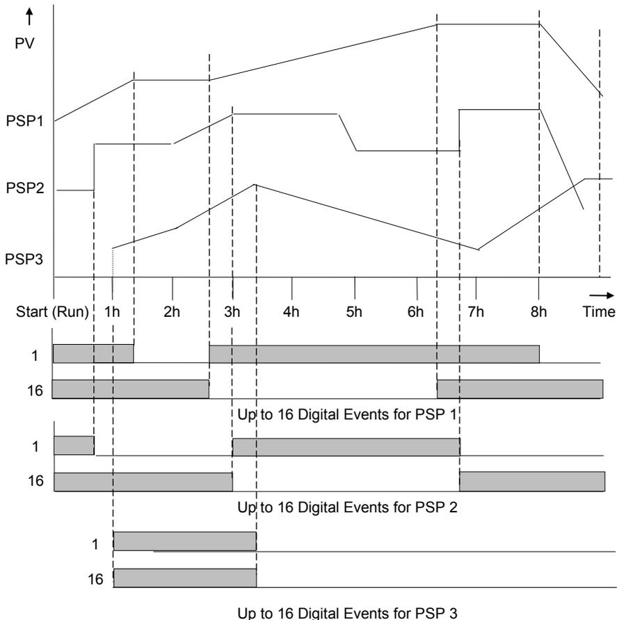
**Figure 4-2: An Example of an Asynchronous Setpoint Program**
