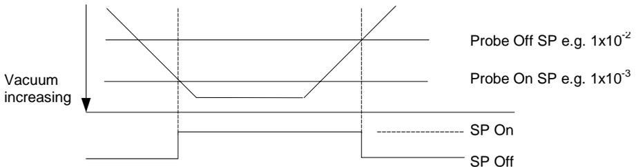
**Figure a-2: Setpoint Output Status when On SP < Off SP**
