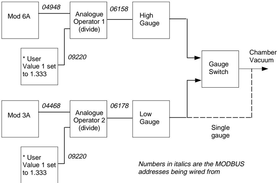
**Figure a-8: Scaling units in a two gauge system**
