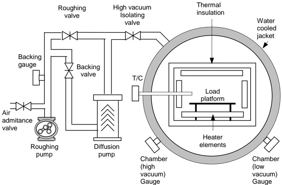
Figure a-1: Representation of a Vacuum Chamber
