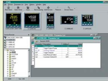
iTools configuration software enables you to store and clone controller configurations, as well as commission your process control system. This facility significantly reduces installation and commissioning time while improving the security of the process. The Eurotherm advanced customer sensor linearisation tool also provides for the download of special sensor response characteristics to the controller.
