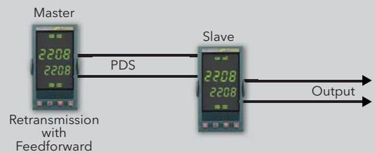
Using Eurotherm setpoint retransmission over PDS communications it is possible to use two 2400 controllers as a cascade control system with the output of the first (or master controller) forming the setpoint of the second (or slave controller).
