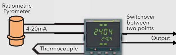
Sometimes it is desirable to control a process using two separate inputs to derive the PV (process value). This could be based on a highest wins, lowest wins, some function of the two inputs, or switching between the two inputs at some pre-determined point in the process.
