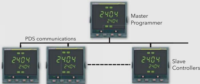
In 2000 Series controllers it is possible to use the PDS communication link to send a setpoint from one controller to a network of slave devices - providing the economical creation of multi-zone temperature control solutions.
