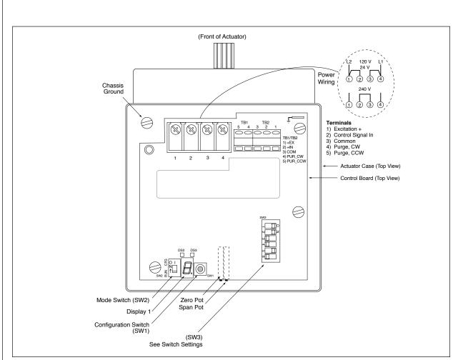
Figure 1. Controller board showing components used during setup and configuration
