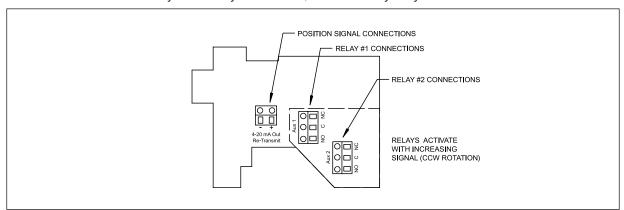
Figure 3. Option board connections
