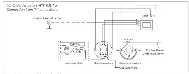
Figure 8. Motor and slidewire for older actuators
