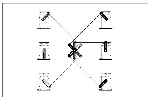
Figure 5. Typical Actuator Mounting Positions
