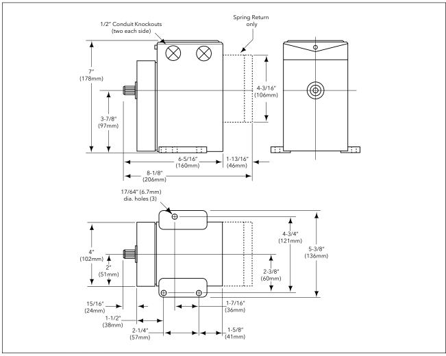
Figure 7. Mounting Dimensions, EA Actuator
