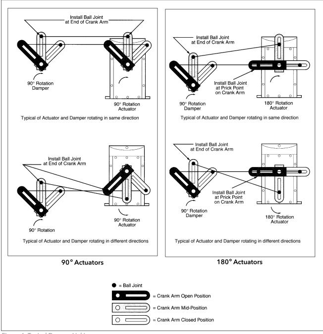
Figure 6. Typical Damper Linking
