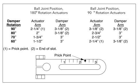
Figure 4. Slot provides adjustment from 7/8" to 3-1/8"
