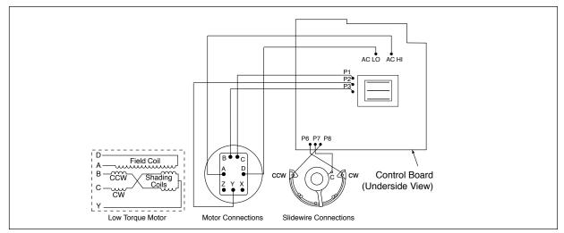
Figure 2. Motor and slidewire connections
